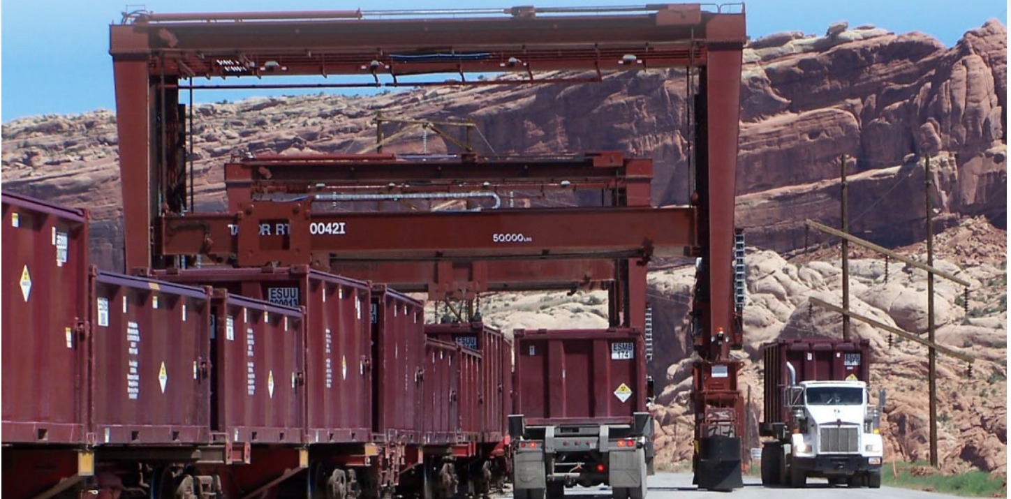
Two gantry cranes at the Moab site transfer containers to and from the train.
