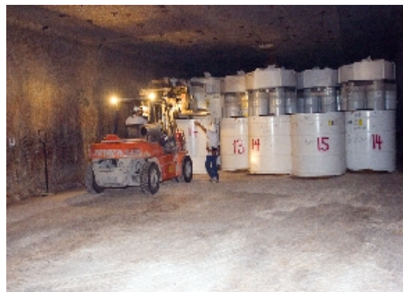
Workers position TRU waste at WIPP.
