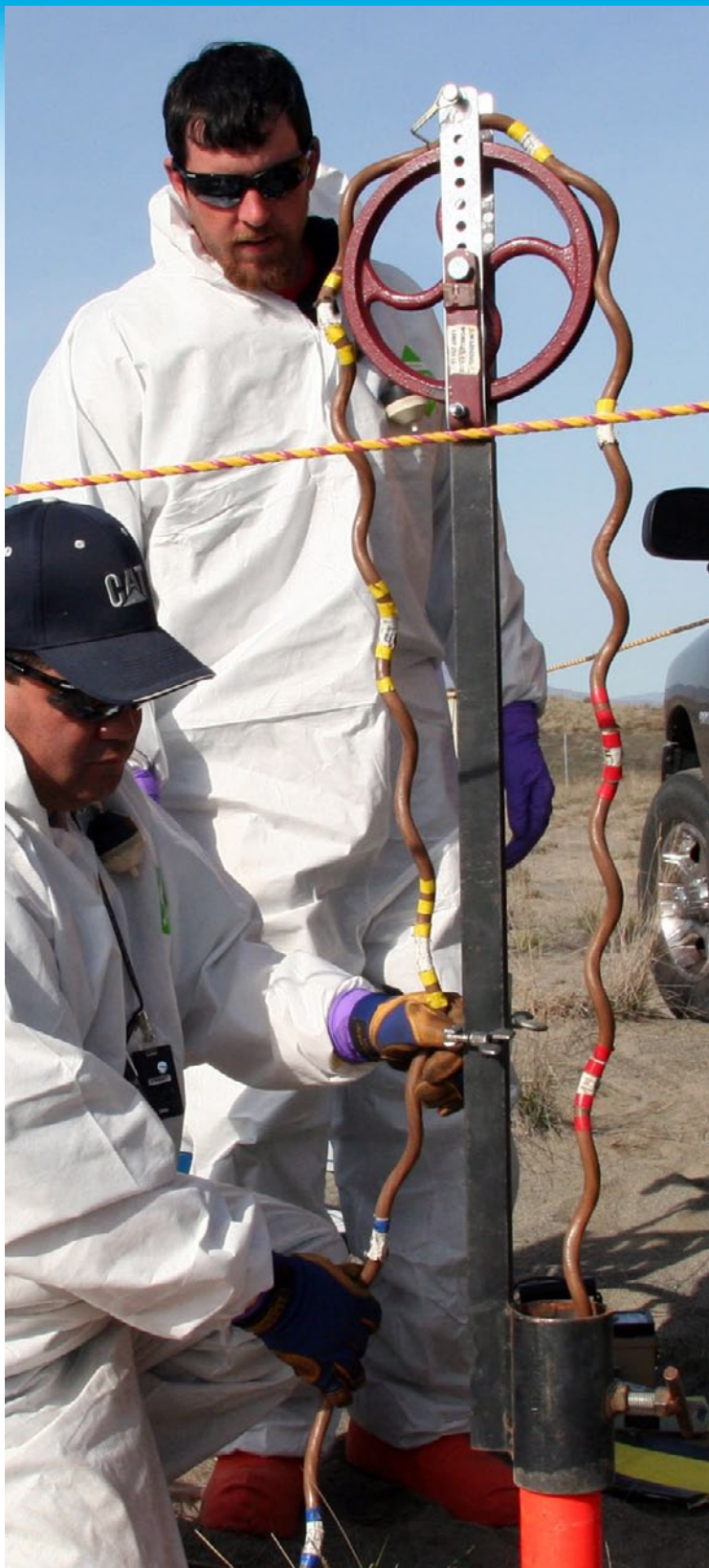
A multi-detector probe is lowered into a narrow steel tube called a cone penetrometer to measure radiation activity at one of the most hazardous waste sites at the Hanford Site.
