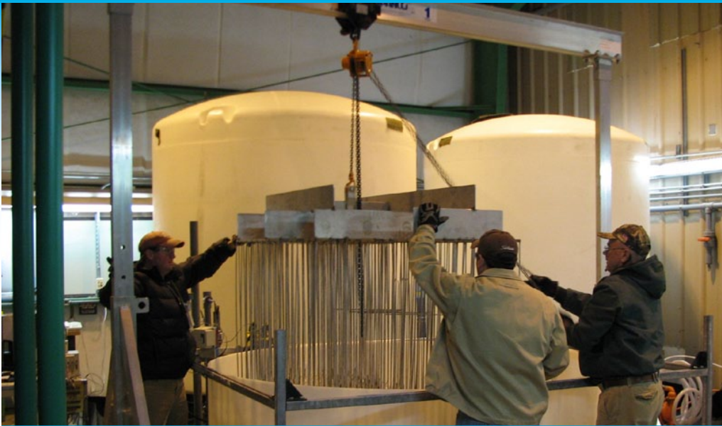
Workers from Savannah River Remediation LLC and the Savannah River National Laboratory designed a scaled-down of an underground waste storage tank, pictured here, to explore how a mixer pump would perform.
