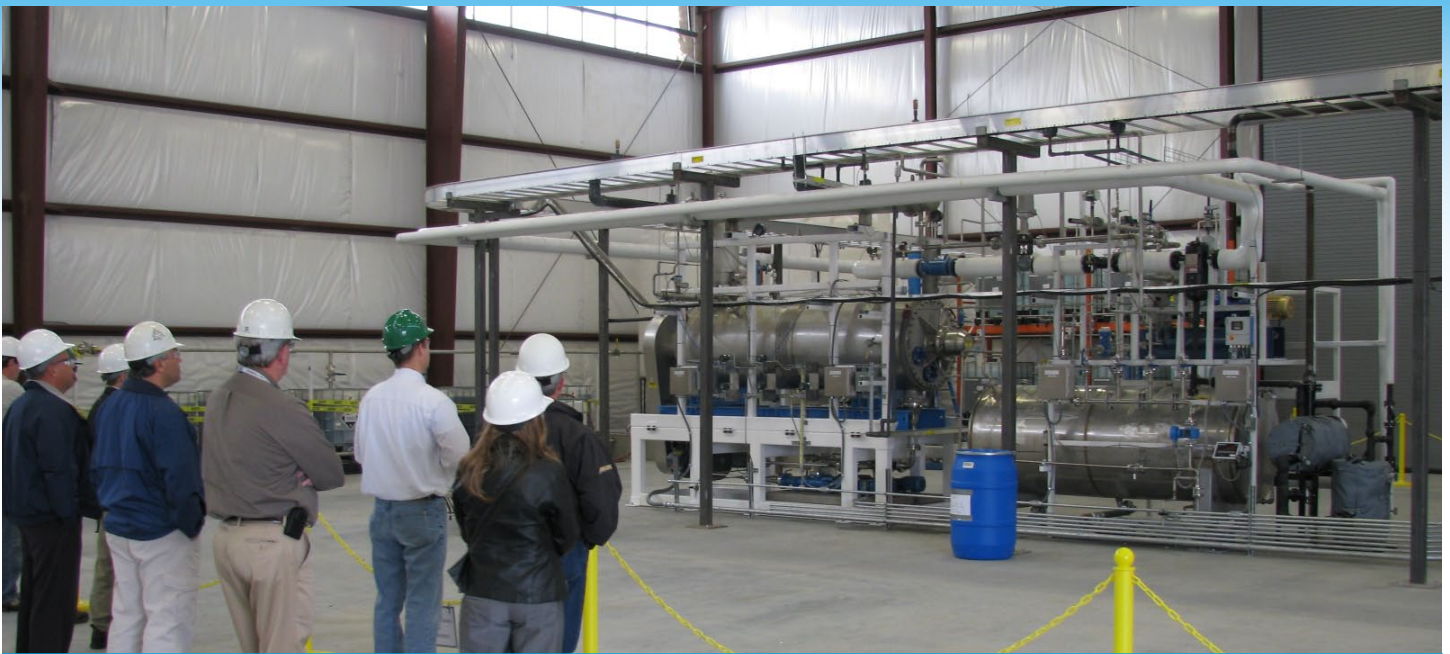
With the help of Recovery Act funding, the Office of River Protection is developing the Wiped Film Evaporator, a new technology offering a portable option for at-tank volume reduction of waste.
