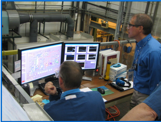
Figure 2. Control Room of Fractional Crystallization Pilot Scale Plant
