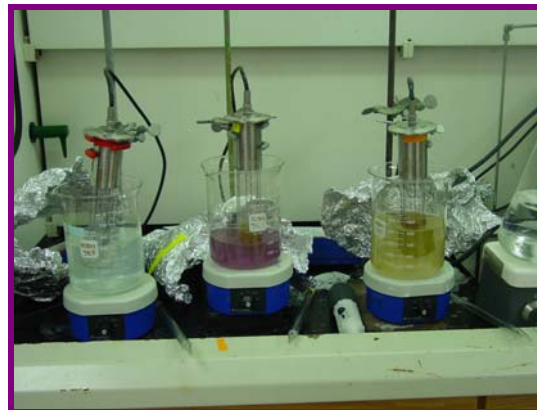
Figure 1: Vacuum Ultraviolet Lamps Used to Simulate Gamma Radiation
