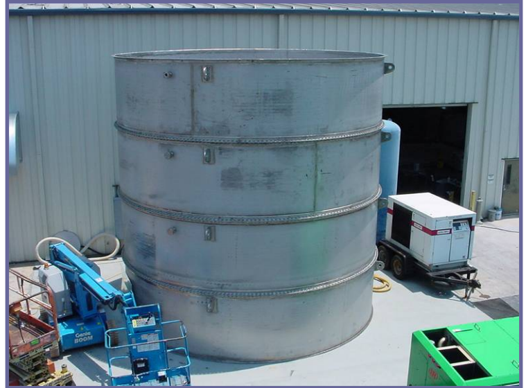
Figure 2. Fabricated Engineering Scale Test Tank
