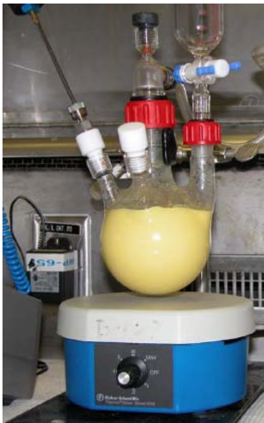
Figure 1. Photograph of Bench-Scale Synthesis of Enhanced Monosodium Titanate (mMST)
