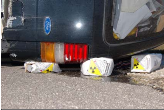
Simulated radioactive material packages are crushed under a rolled delivery van
