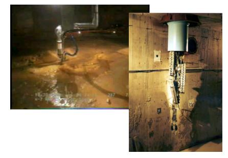
Waste retrieval equipment utilized today has little ability to control properties of the resulting slurries that are conveyed out of the tanks.
