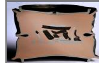
Metal encapsulation of uneconomic feeds (Swedish SNF in copper shown)
