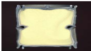
Cold calcine in glass-ceramic matrix
