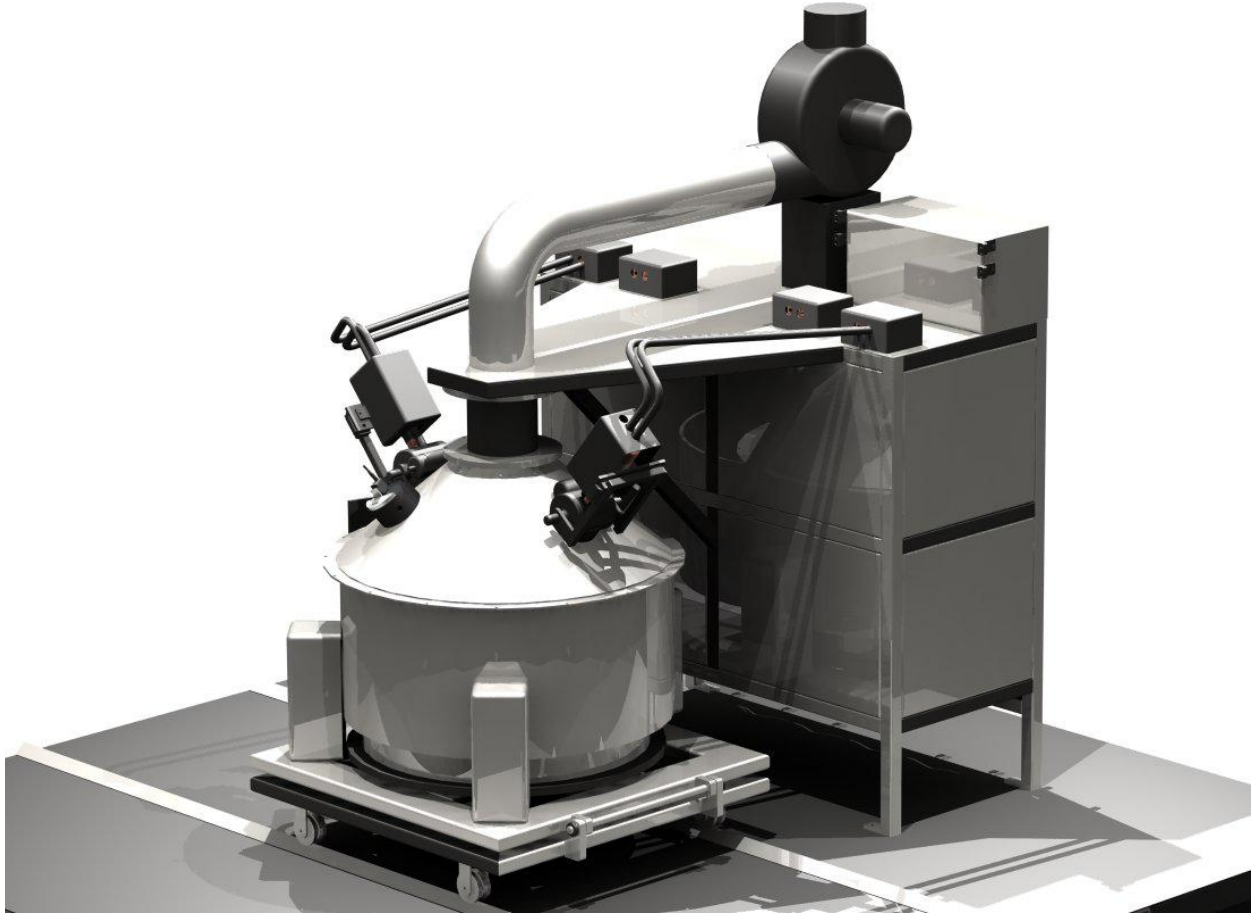
Figure 8-7. Solidworks® Drawing of Plasma Arc Melter
