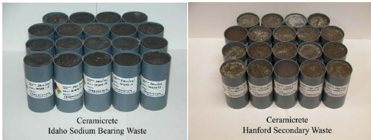
Figure 6-12. Chemically Bonded Phosphate Ceramics Proposed for INL and Hanford Wastes [50]
