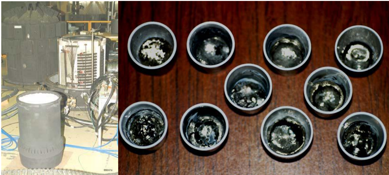
Figure 6-11. Metal Waste Form Production Furnace being readied for Installation [48] and a Zirconium-based Metallic Waste Form (right) [47]
