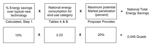
**Step 5:** To obtain the related carbon emission savings for the 0.045 quads, look up the appropriate generic carbon emissions factor in Table C. The conversion value is 16.33 MMTC/quad (million metric tonnes of carbon per quad of primary energy). Insert the two values into the boxes, and multiply the energy savings by the conversion factor. The result is a 0.73 million metric tonne reduction of carbon emissions.
