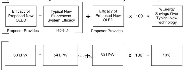
proposer establishes that the product has a system efficacy of 60 lumens per watt. Convert that performance into a % energy savings over typical new fluorescent systems. Compared to a typical new fluorescent system of 54 lumens per watt, the proposed OLED is 10% more efficient.
