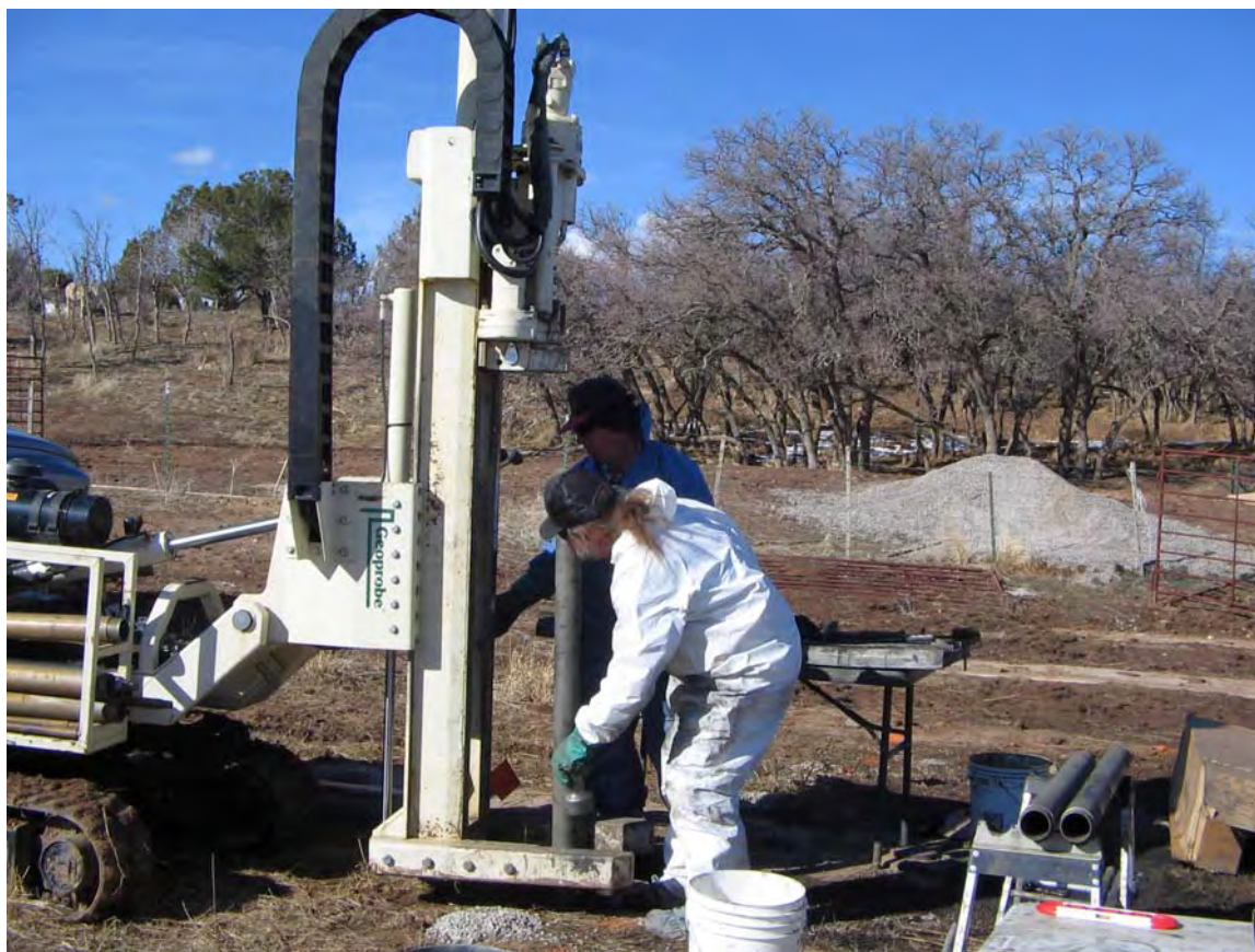
Figure 3. Photo of Geoprobe Rig Obtaining a Core
