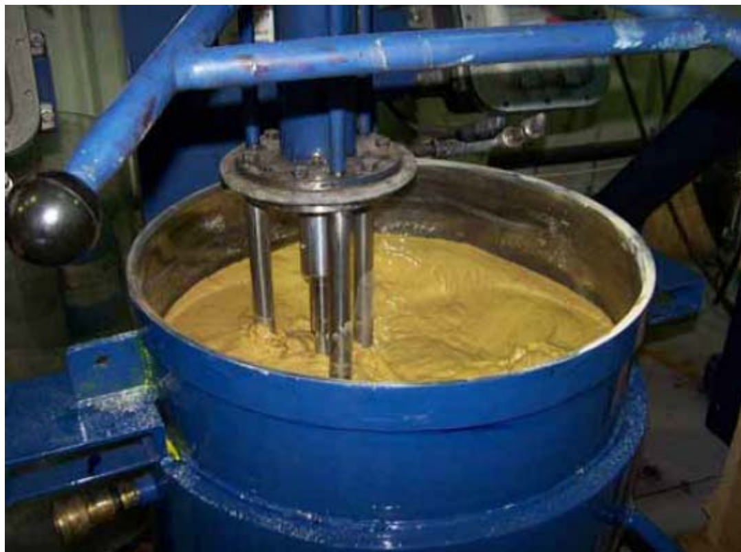
Figure 3-10. Slurry of ground CST at 40% solids. The process will be operated at 20% solids for transport ease. The slurry is pumpable to Tank 40
