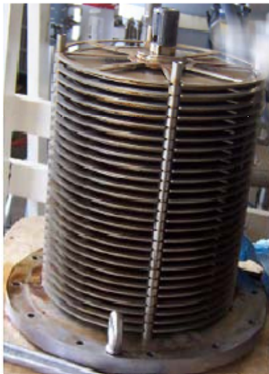
Figure 3-4. Full scale, 25-disk Filter used in test activities
