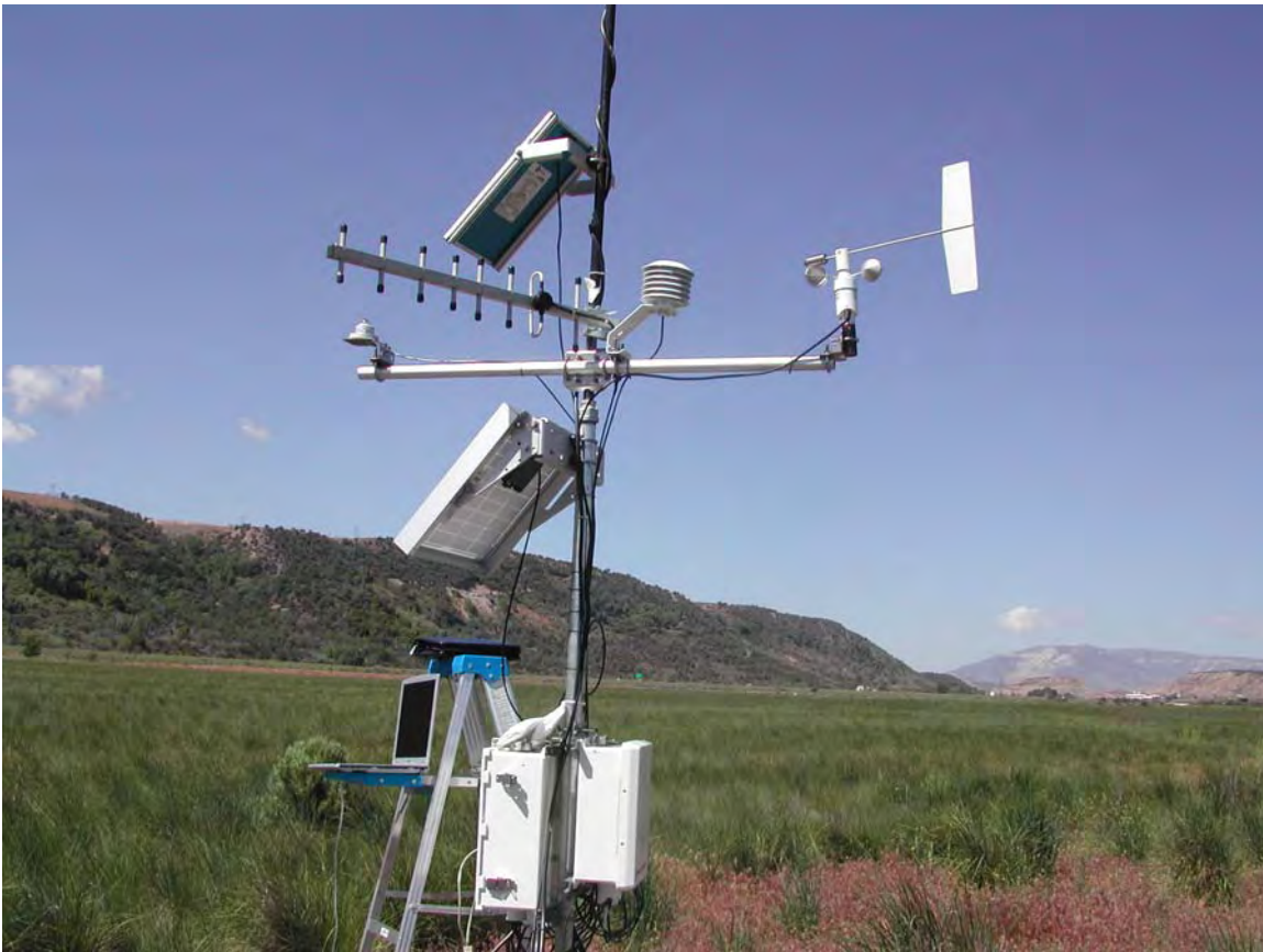
Figure 6. SOARS Station at Well 0857, Collects Data from Well 0857 and Weather Instruments
