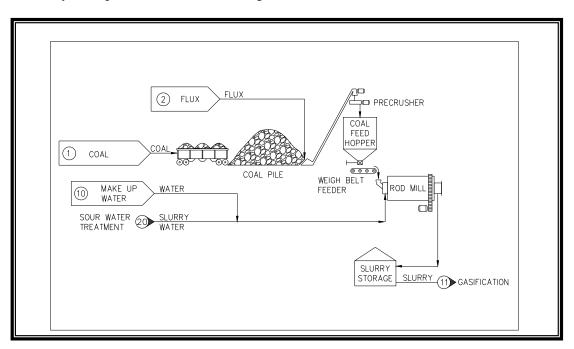
Figure 2.2-3. Feedstock Grinding and Slurry Preparation
