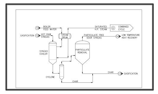
Figure 2.2-5. Particulate Matter Removal
