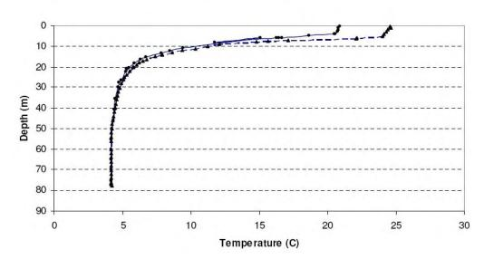
Figure 4.5-5. Temperature Profiles for the Canisteo Mine Pit Using 2006 Data (Barr, 2008b)
