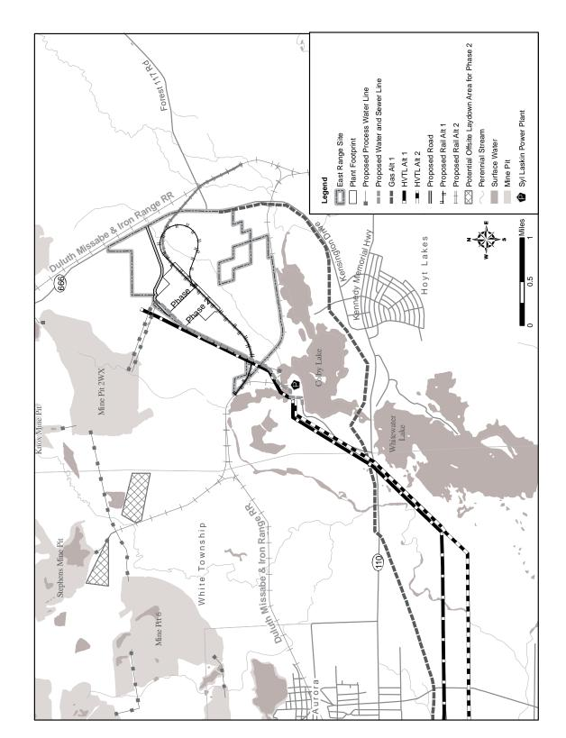
The CN operates trains daily on the track serving Minnesota Power's Syl Laskin Generating Station. Coal would be delivered by other railroads to the CN at either Superior, Wisconsin, or at a rail yard south of Eveleth, Minnesota. The CN rail line would be used to deliver coal to the site from Eveleth, and empty trains would return by the same route.
