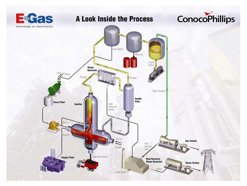
Figure 2.2-2. E-Gas™ Process for IGCC Power Generation
