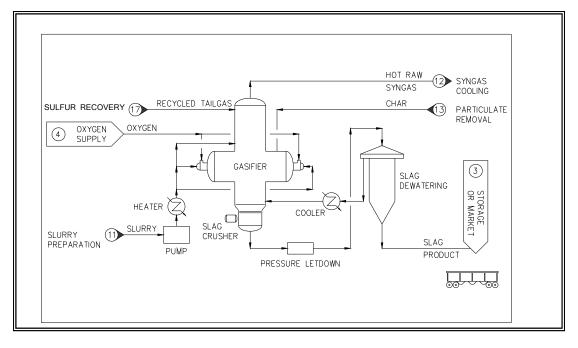
Figure 2.2-4. Gasification and Slag Handling
