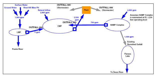
Figure 4.5-3. Phase I Water Balance: West Range IGCC Power Station (revised in Final EIS)
