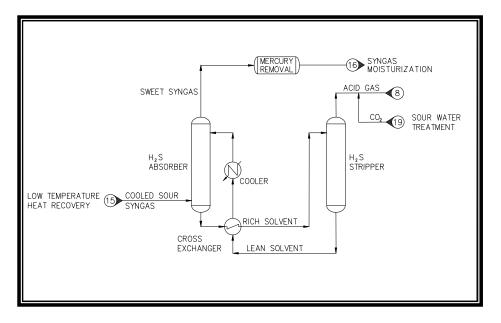
Figure 2.2-7. Acid Gas Removal and Mercury Removal
