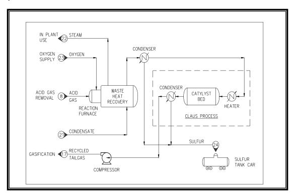
Figure 2.2-8. Sulfur Recovery Unit
