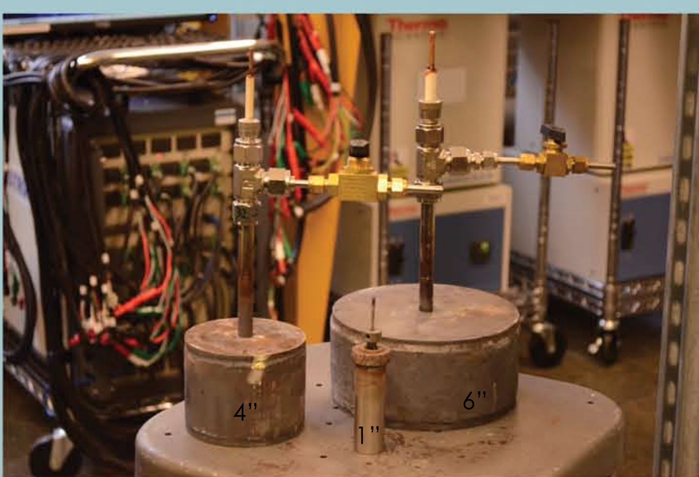
Figure 6. Initial testing took place at the 1Ah scale (center). Cells have now been scaled to 20Ah and 200Ah (left & right).
