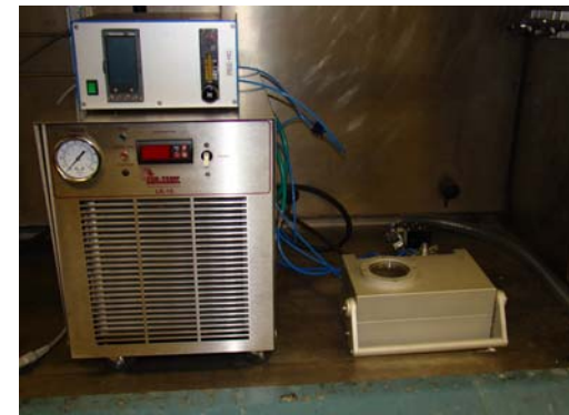
Vacuum Solder Reflow System for processing void-free joints
