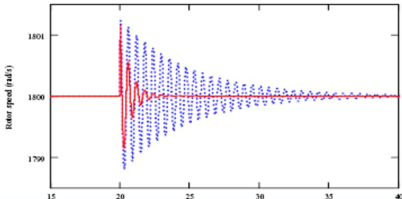
Optimal feedback gains control (from LQR program) of energy storage device
