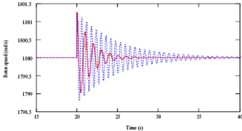
Lag compensator control of energy storage device
