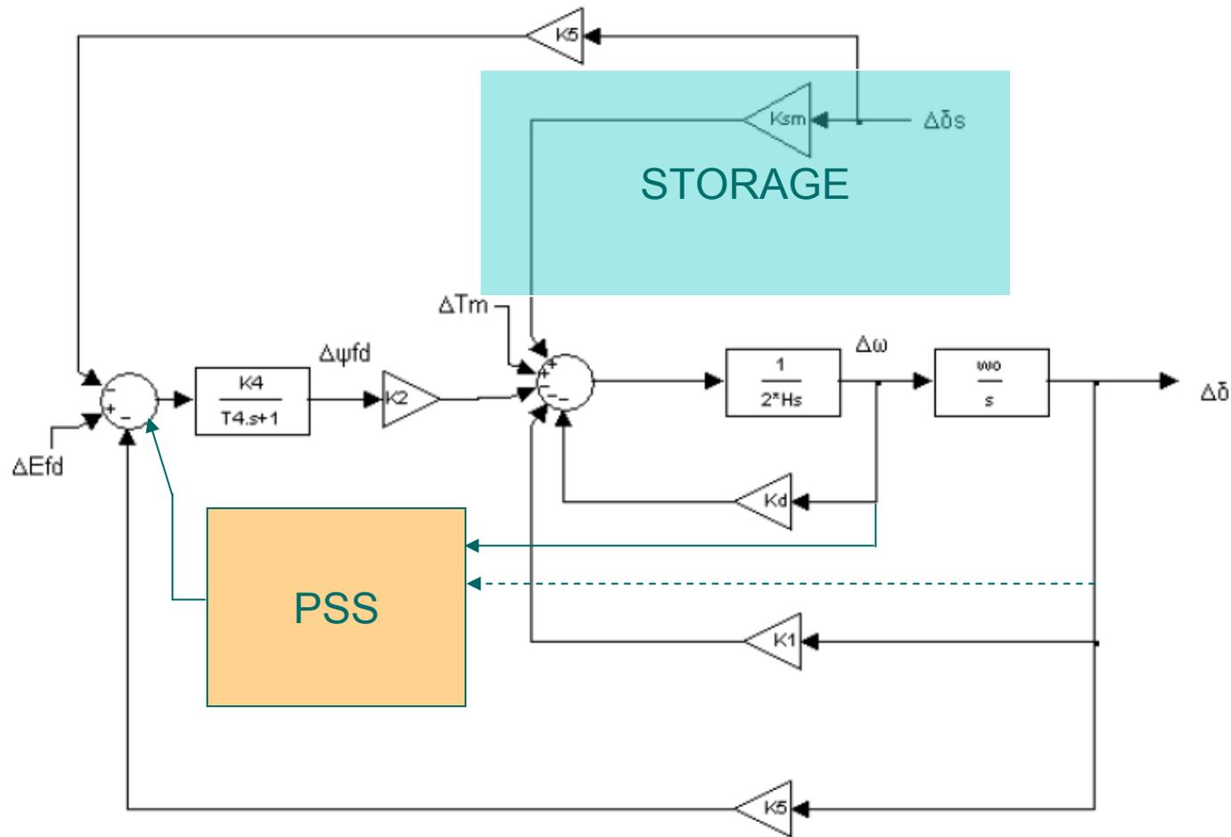
Block diagram shows classical PSS feedback path through field and more direct ESS feedback path
