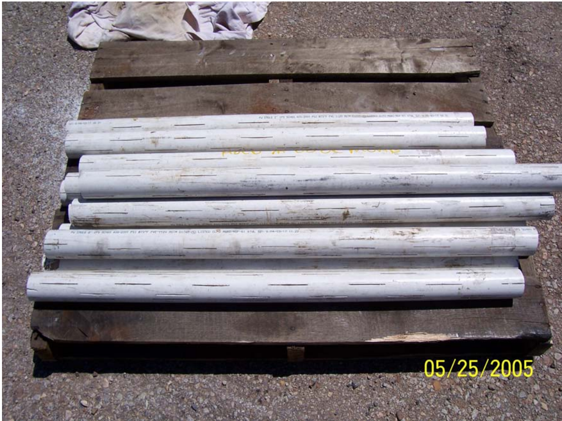
Figure 14. Piping used for distribution (bottom of cell) and collection (top of cell) networks. Two-inch schedule 80 PVC pipe with 0.080-inch-wide slots.
