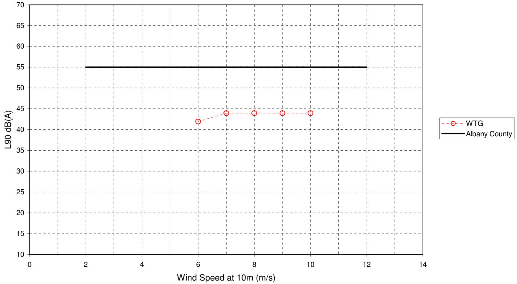
Location 6: Siemens SWT 2.3mW Turbines - 24 Hour Data
