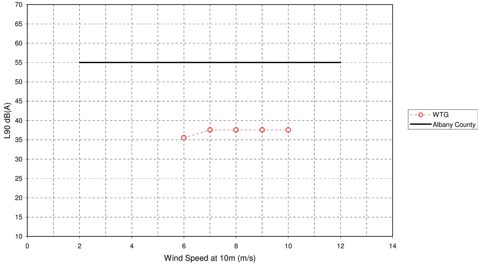
Location 15: Siemens SWT 2.3mW Turbines - 24 Hour Data
