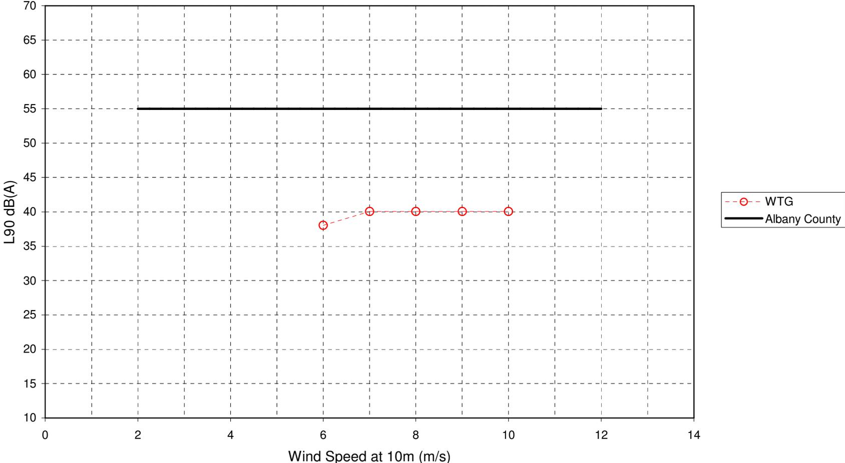
Location 9: Siemens SWT 2.3mW Turbines - 24 Hour Data
