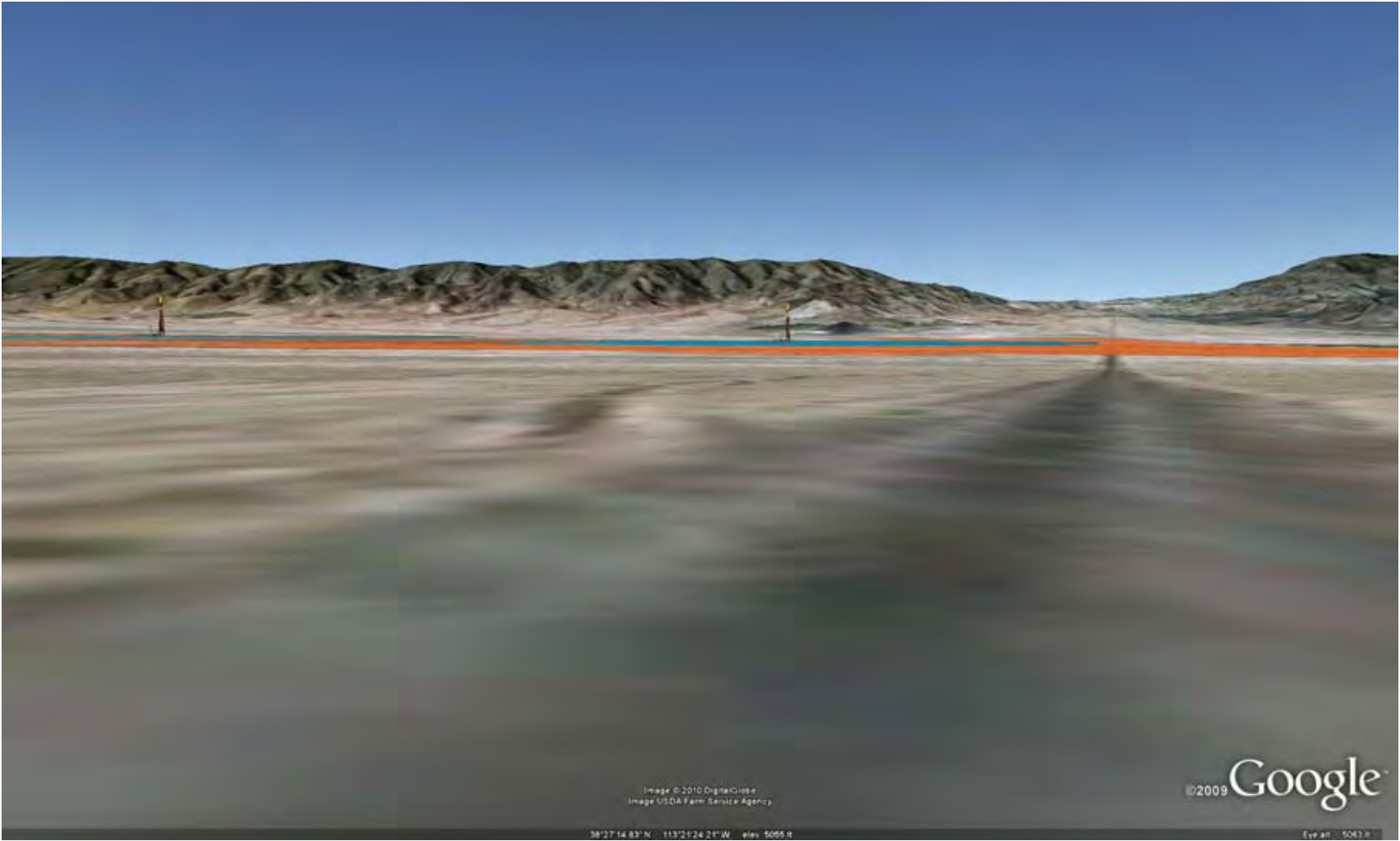
FIGURE 13.3.14.2-6 Google Earth Visualization of the Proposed Wah Wah Valley SEZ (shown in orange tint) and Surrounding Lands, with Power Tower Wireframe Models, as Seen from State Route 21 Approximately 1.4 mi (2.3 km) East of the SEZ
