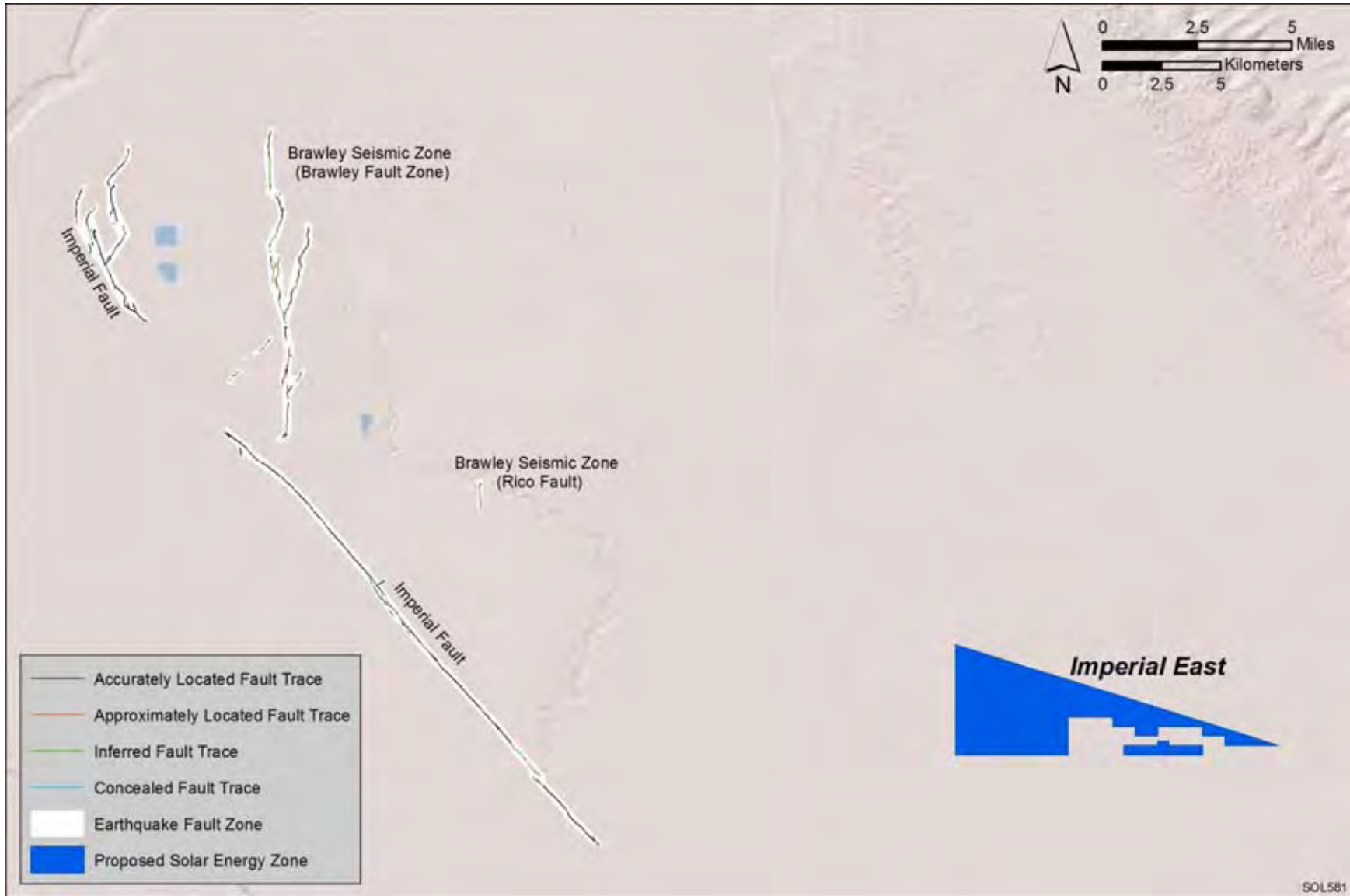
FIGURE 9.1.7.1-5 Delineated Earthquake Fault Zones near the Proposed Imperial East SEZ (CGS 2010)
