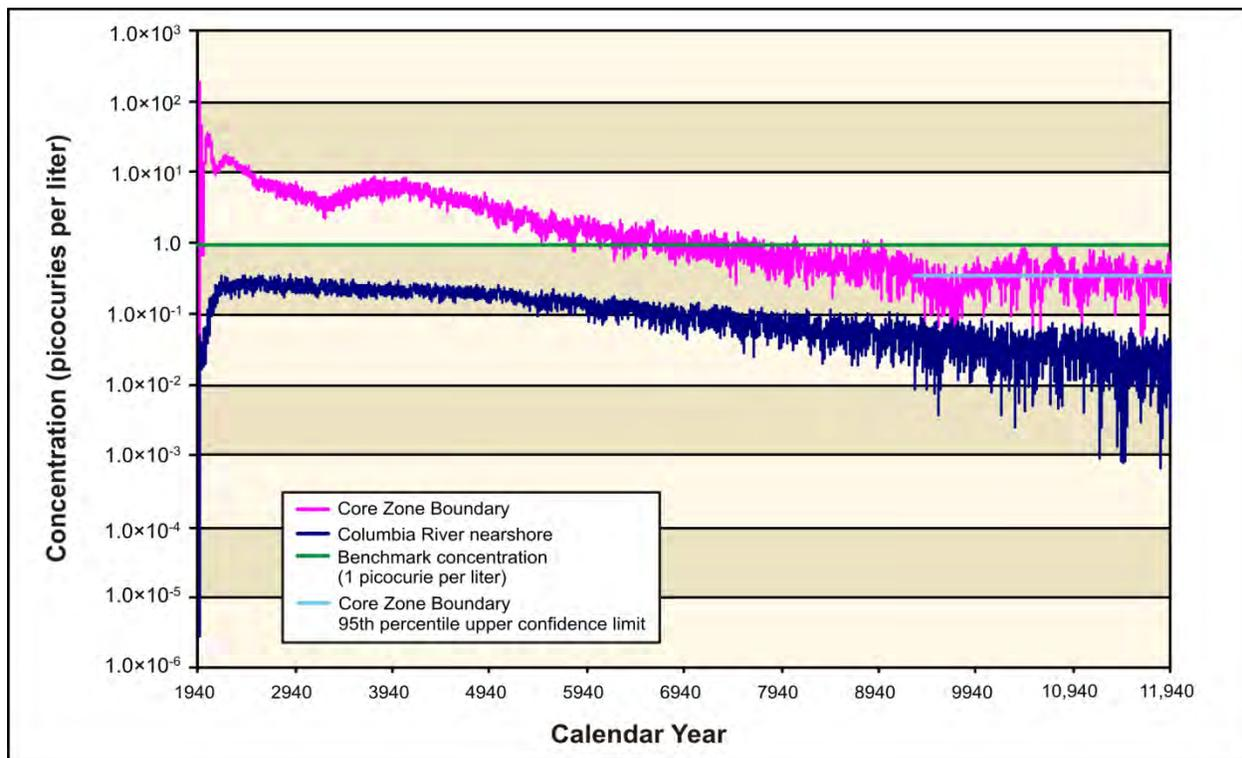
Figure 23. Tank Closure Alternative 2B Iodine-129 Concentration Versus Time
