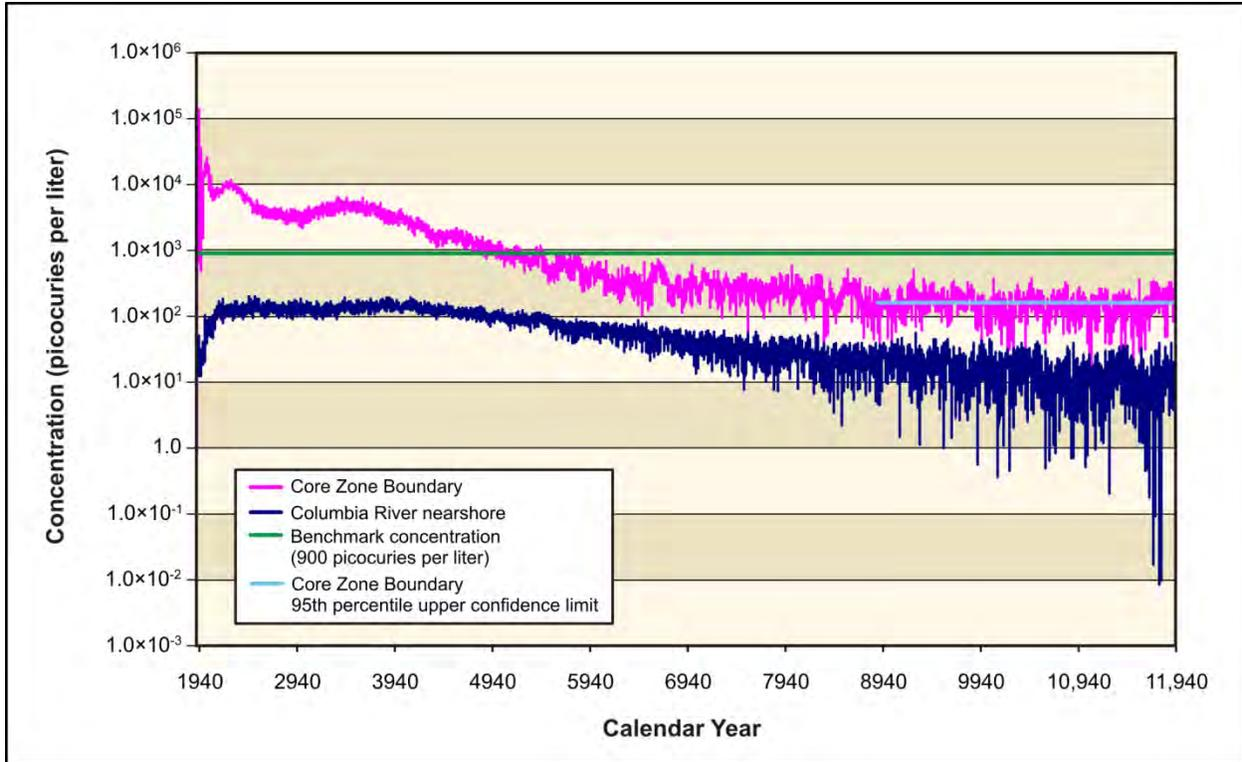
Figure 24. Tank Closure Alternative 2B Technetium-99 Concentration Versus Time
