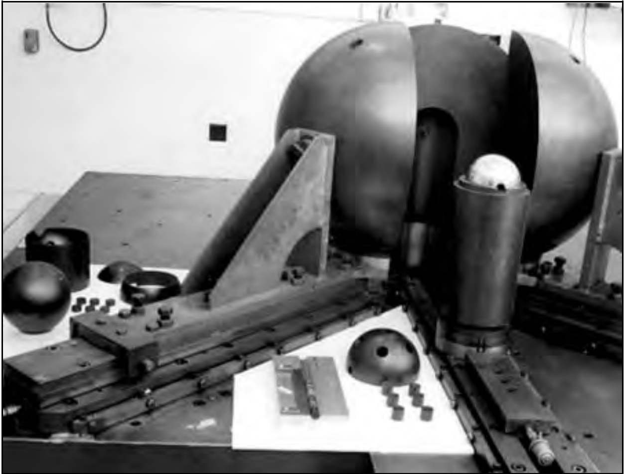
Figure A-1 Flattop Benchmark Assembly
