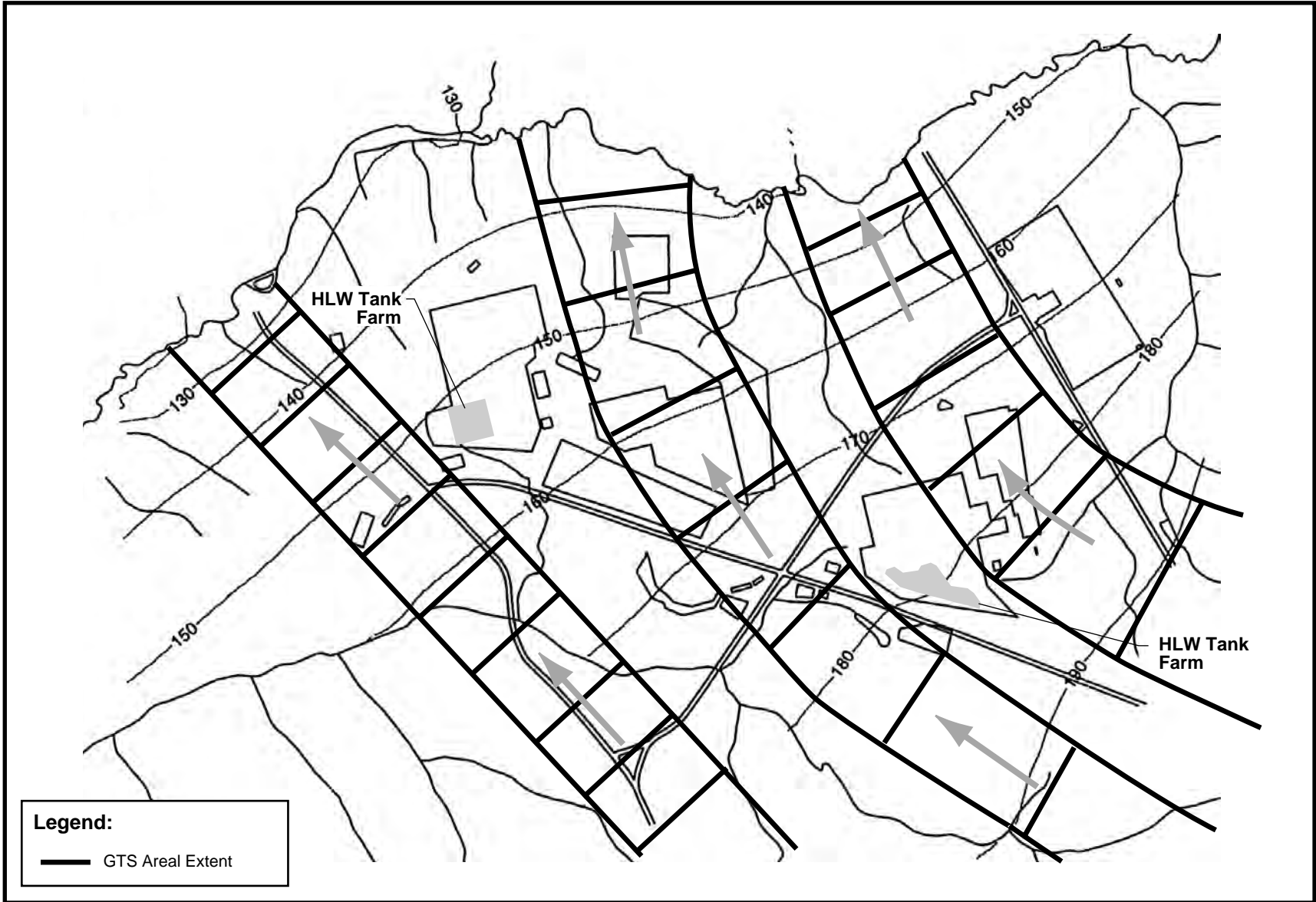
Figure 3.2-4. Calibrated potentiometric surface (ft) for the Congaree aquifer.
