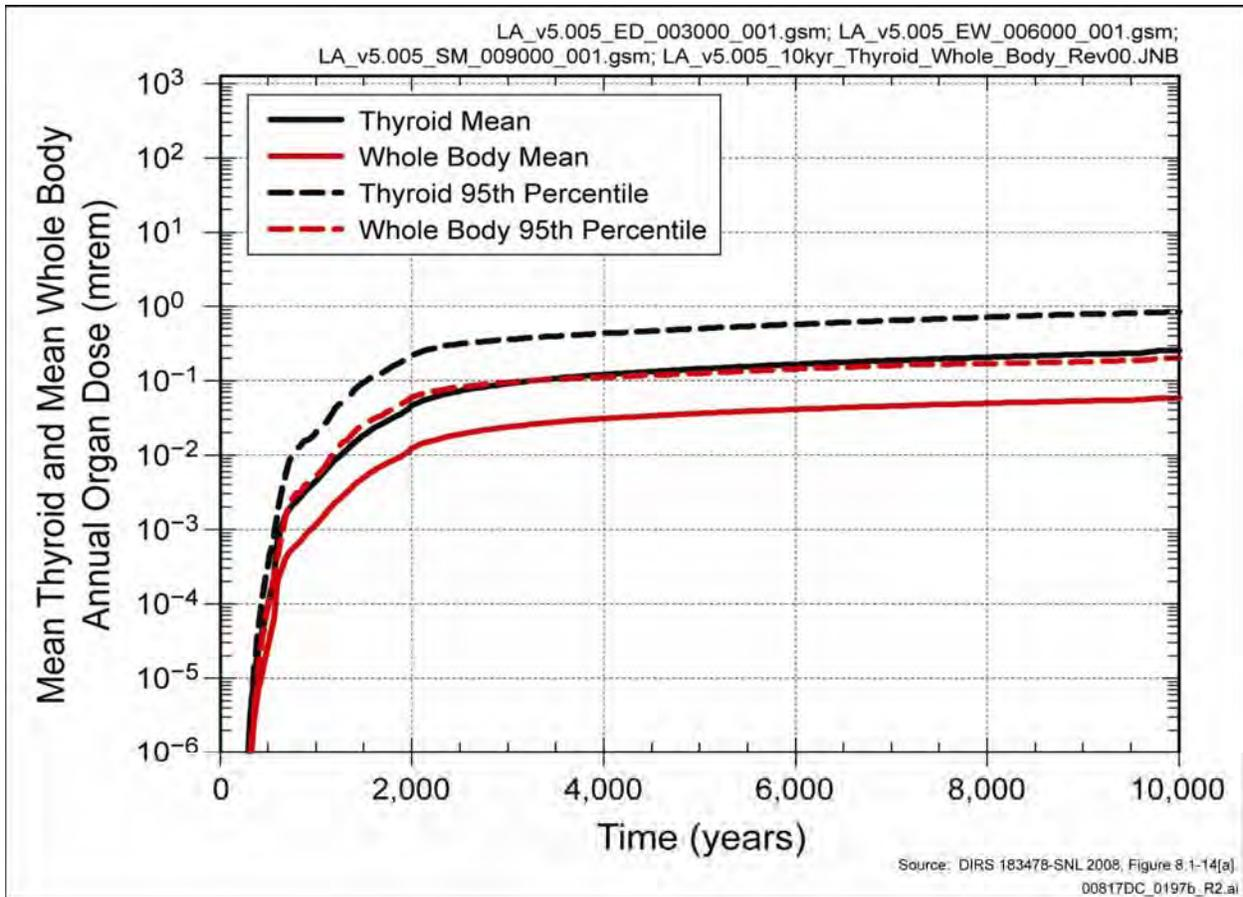
**Figure F-20.** Mean annual drinking water dose from combined beta and photon emitters for likely features, events, and processes using the nominal, early failure, and seismic ground motion damage processes.
