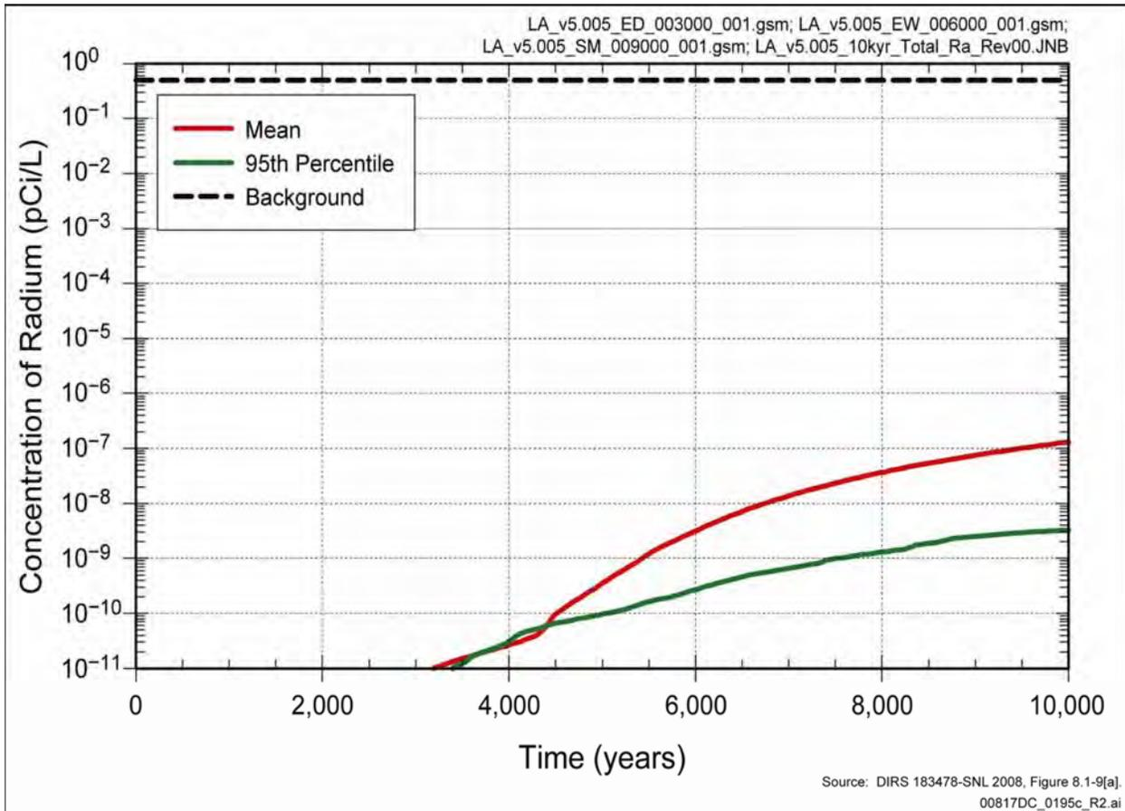
**Figure F-18.** Combined radium-226 and -228 activity concentrations, excluding natural background, for likely features, events, and processes using nominal, early failure, and seismic ground motion damage processes.
