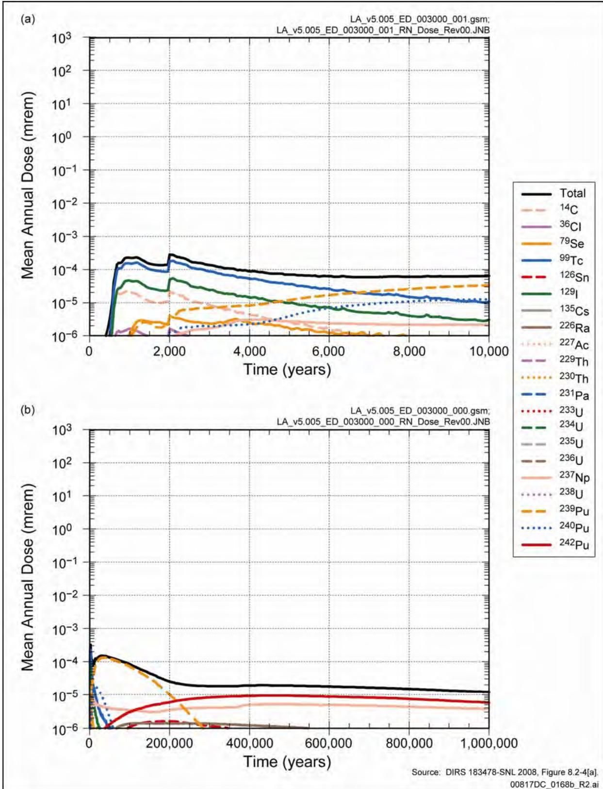
**Figure F-6.** Mean annual dose histories of major radionuclides for the Drip Shield Early Failure Modeling Case for (a) the first 10,000 years after repository closure and (b) the post-10,000-year period.
