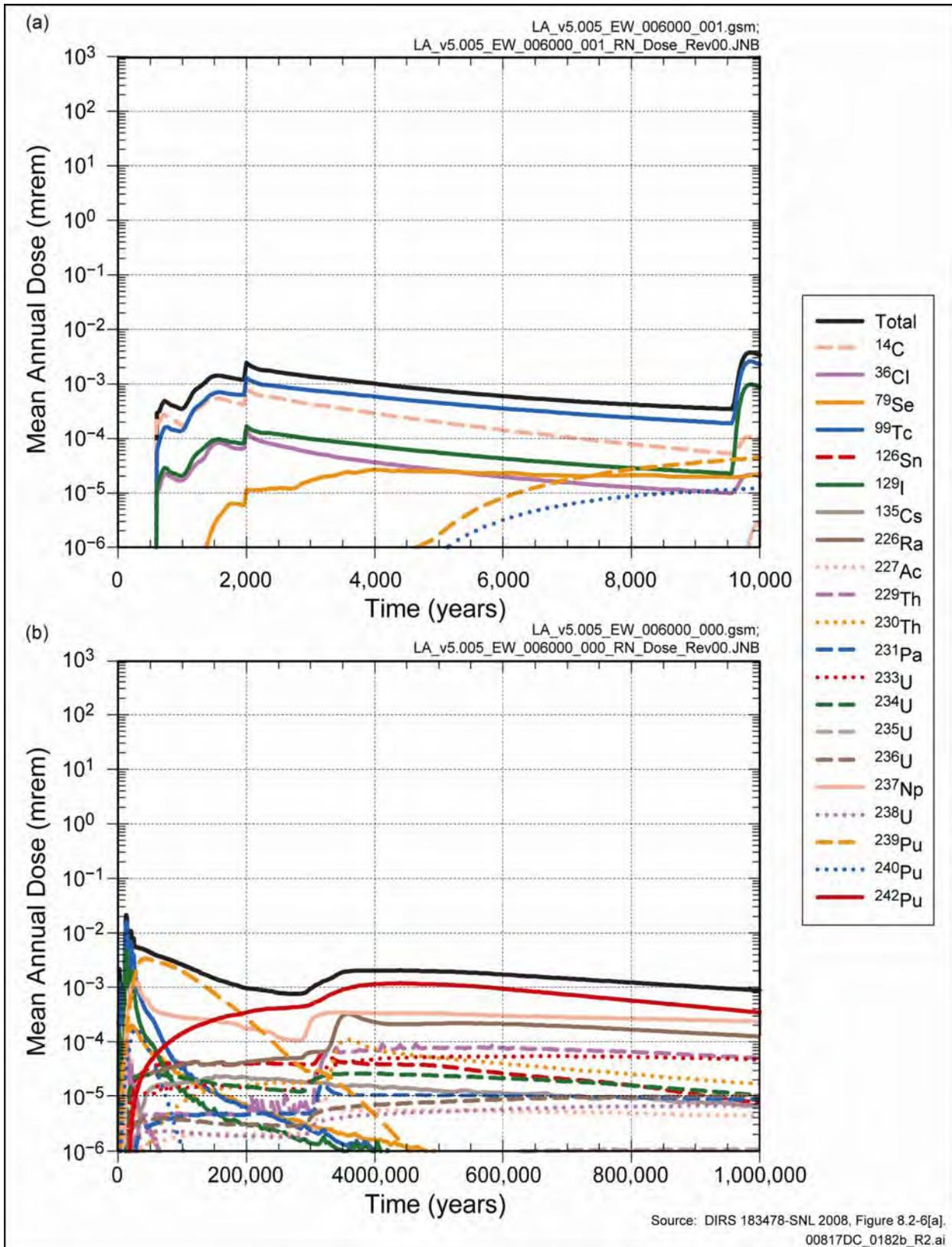
**Figure F-8.** Mean annual dose histories of major radionuclides for the Waste Package Early Failure Modeling Case for (a) the first 10,000 years after repository closure and (b) the post-10,000-year period.
