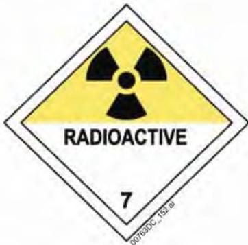
**Figure H-2.** Radioactive hazard communication placard.
