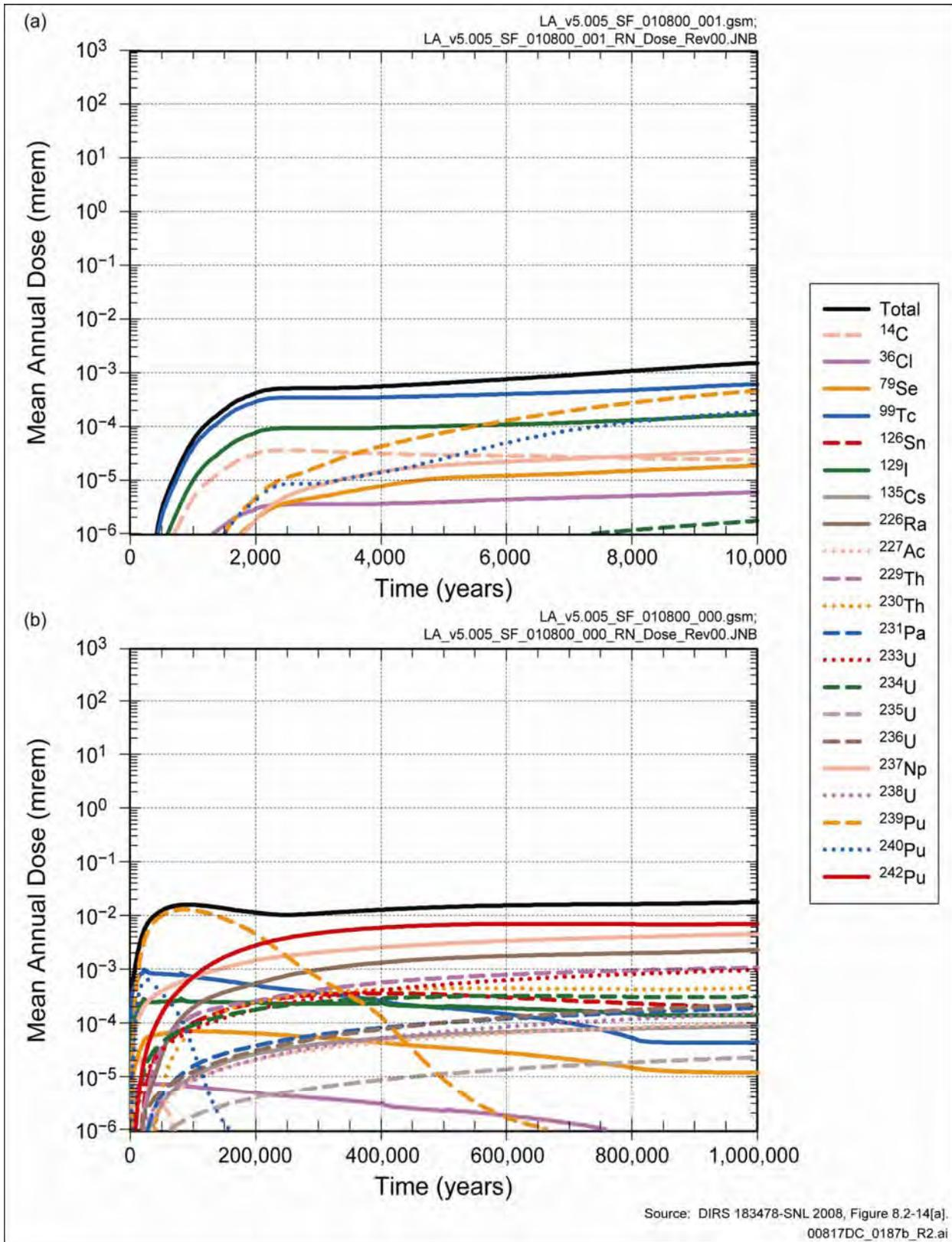
**Figure F-16.** Mean annual dose histories of major radionuclides for the Seismic Fault Displacement Modeling Case for (a) the first 10,000 years after repository closure and (b) the post-10,000-year period.
