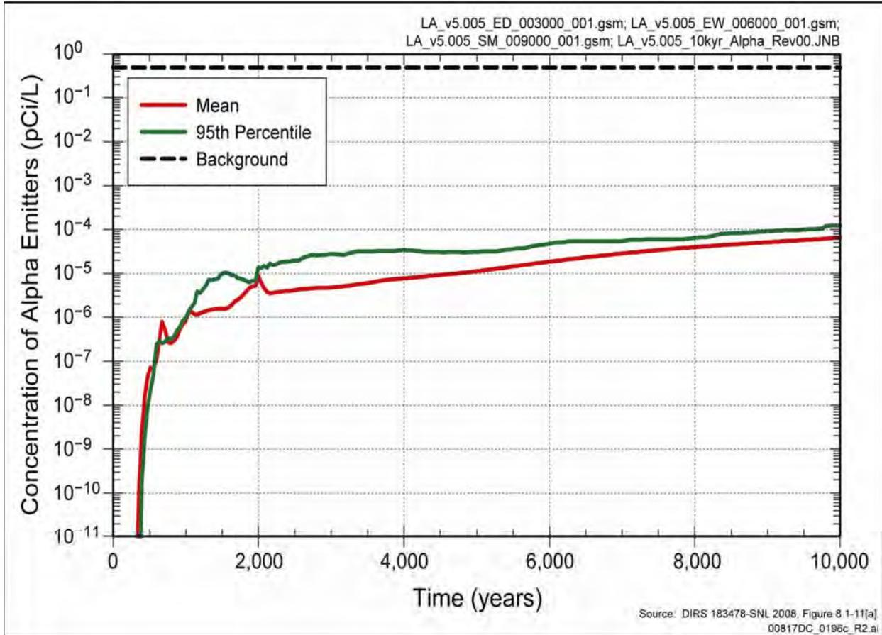
**Figure F-19.** Combined activity concentrations of all alpha emitters (including radium-226 but without radon and uranium isotopes), excluding natural background, for likely features, events, and processes using nominal, early failure, and seismic ground motion damage processes.
