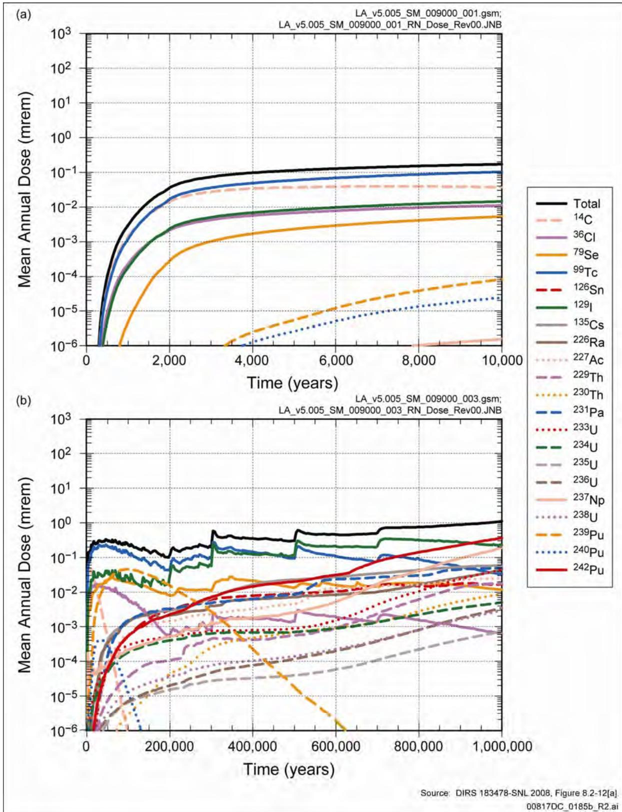
**Figure F-14.** Mean annual dose histories of major radionuclides for the Seismic Ground Motion Modeling Case for (a) the first 10,000 years after repository closure and (b) the post-10,000-year period.
