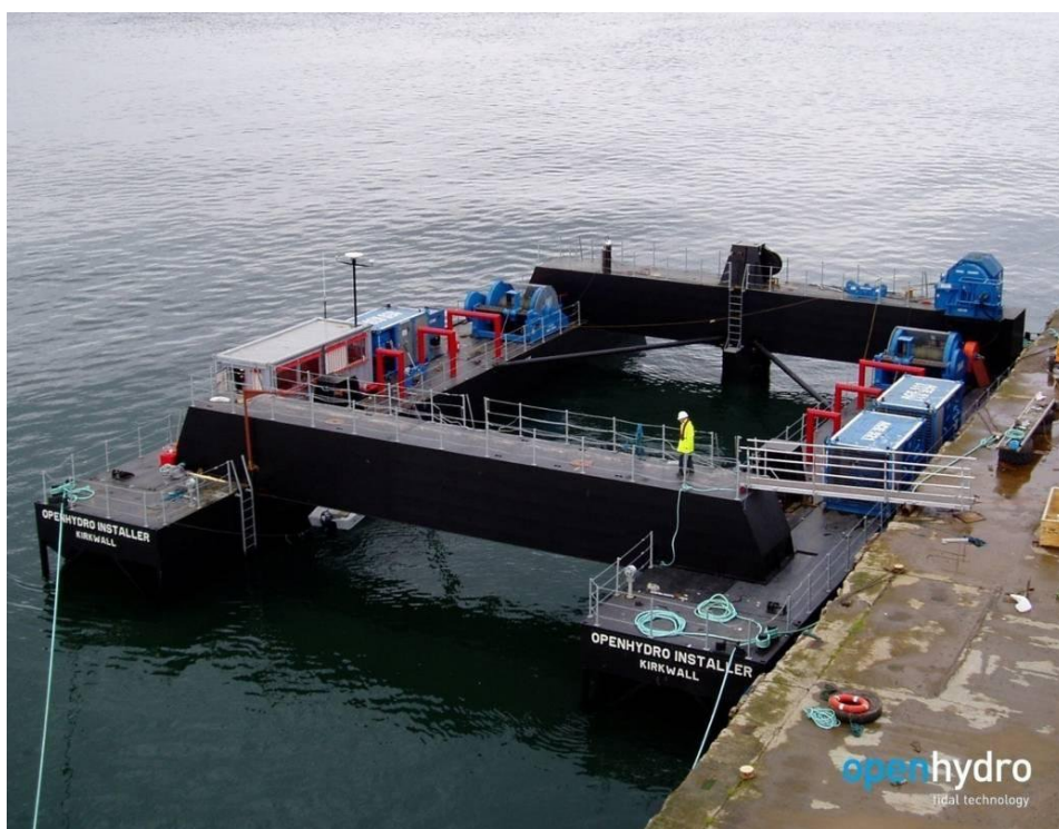
Figure 3. OpenHydro Installation Barge (Source: application).
