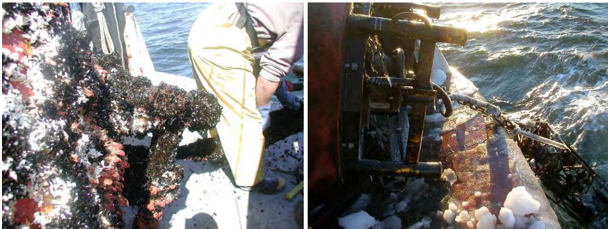
Figure 3-14. Representative Biofouling on Gulf of Maine Oceanographic Buoys
