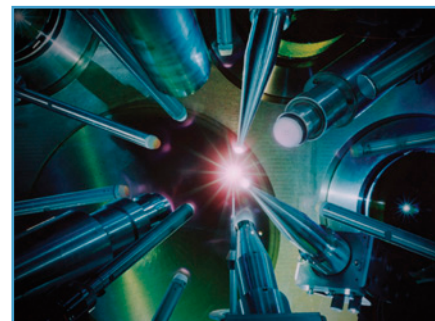
The international inertial confinement fusion community uses the OMEGA laser at the University of Rochester's Laboratory for Laser Energetics to conduct experiments and test target designs and diagnostics.
