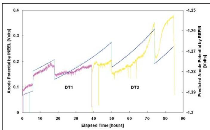
Figure 2. Anode potential comparison for two runs in repeatability tests by REFIN.
