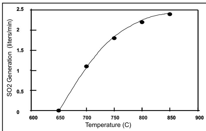
Figure 3. SO<sub>2</sub> generation rate as a function of peak (external) temperature in the SiC bayonet heat exchanger.
