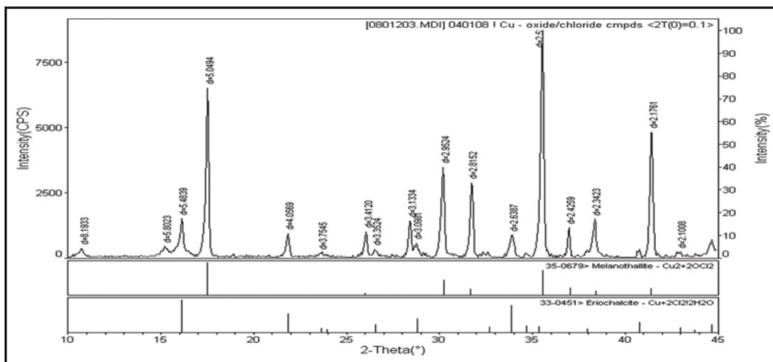
Figure 1. XRD pattern for a product of the hydrolysis reaction using a nebulizer reactor.
