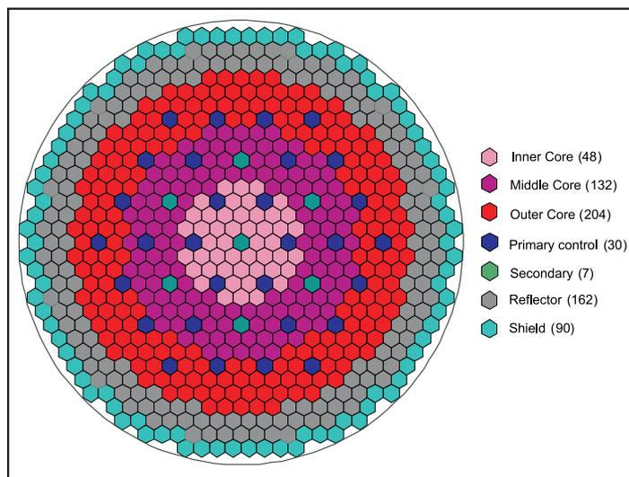
Figure 1. Radial Layout of 2,000-MWth Core Concept.
