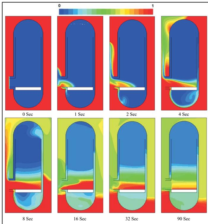
Figure 1. Variations of air distributions in the reactor core during stratified flow.
