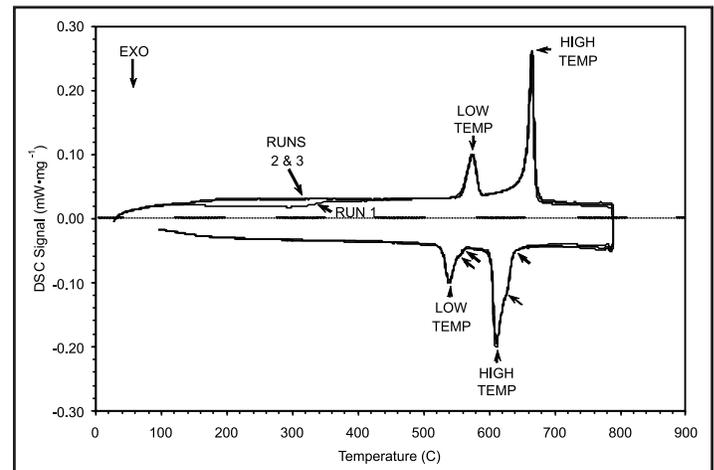
Figure 3. Heating and cooling traces obtained from the differential scanning calorimetry/DTA measurements on an AFC-2 irradiation test series fuel sample.
