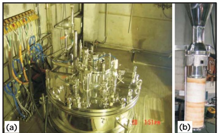
Figure 2. Modified engineering-scale equipment for electrolytic reduction of oxide fuels in KAERI's ACP: (a) top flange and (b) cathode.
