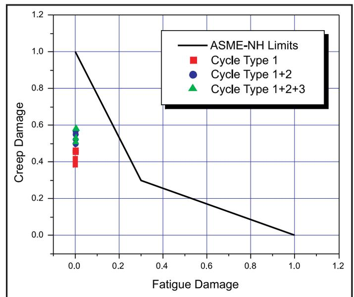
Figure 2. Results of creep-fatigue evaluation for selected ABTR duty cycle events for modified ABTR preconceptual design: Type 1 = Heat-up from hot standby to full power and cool-down to hot standby with hold at full power; Type 2 = Heat-up from refueling to full power and cool-down to refueling with hold at full power; Type 3 = Daily load following.
