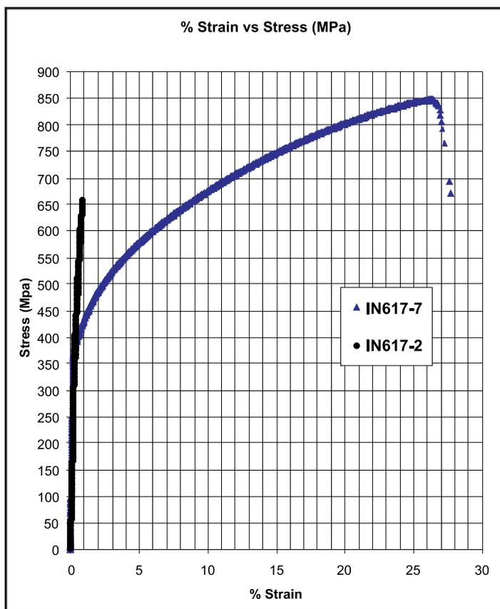
Figure 2. Room temperature tensile stress-strain curves for Inconel 617 that has been oxidized (IN617-7) and carburized (IN617-2) at 900°C for 1,000 hours.
