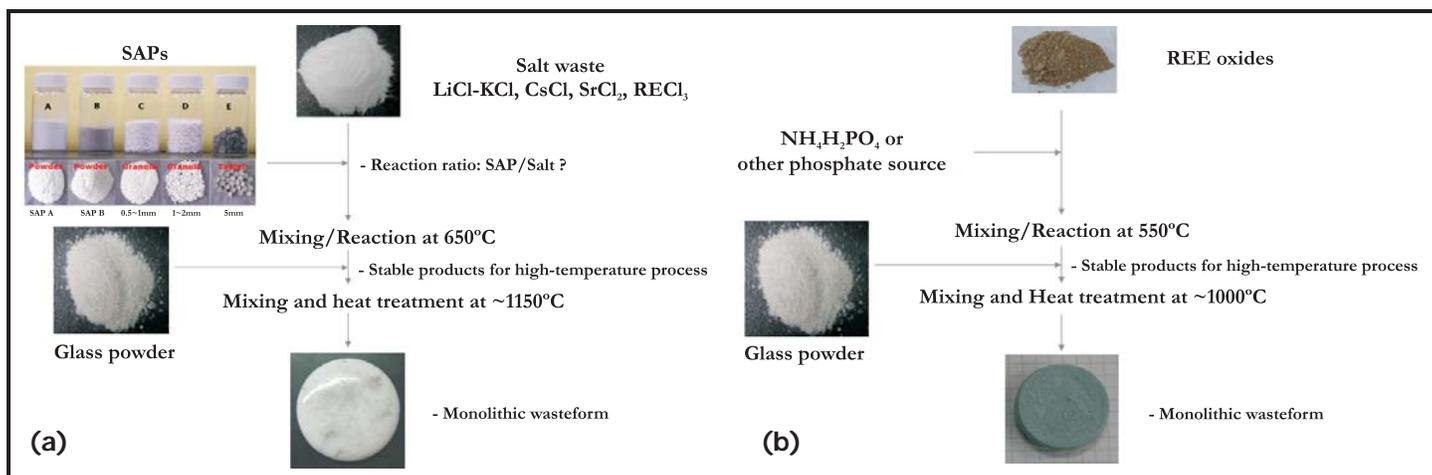
Figure 1. Immobilization procedure for the expected wastes: (a) salt waste and (b) RE oxide waste.
