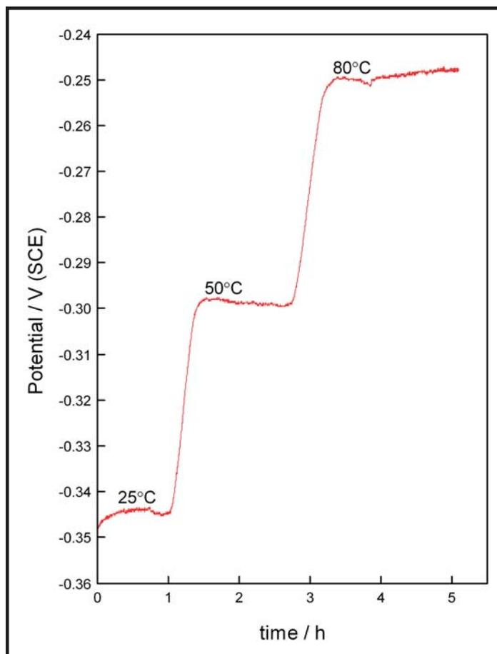
Figure 2. Potential of the hydrogen production reaction during constant-current electrolysis at the temperatures indicated. The current density was 100 mA/cm<sup>2</sup>. The working electrode was 20 percent Pt/XC-72R on a graphite plate working electrode.
