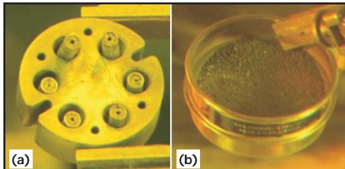
Figure 1. (a) Irradiated MOX fuel sections and (b) crushed and sieved MOX fuel particles.
