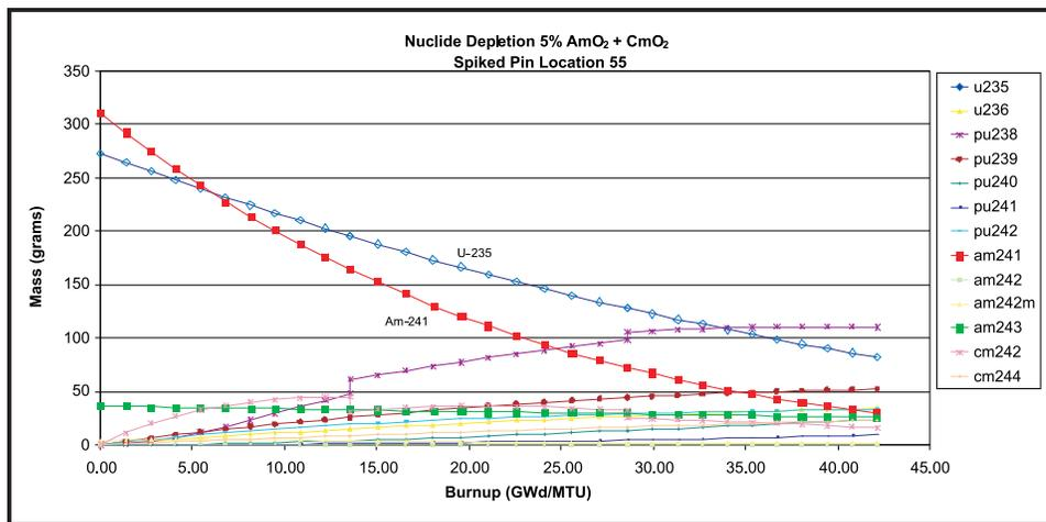
Figure 1. Depletion of  $^{241}\text{Am}$  and other nuclides in PWR application.
