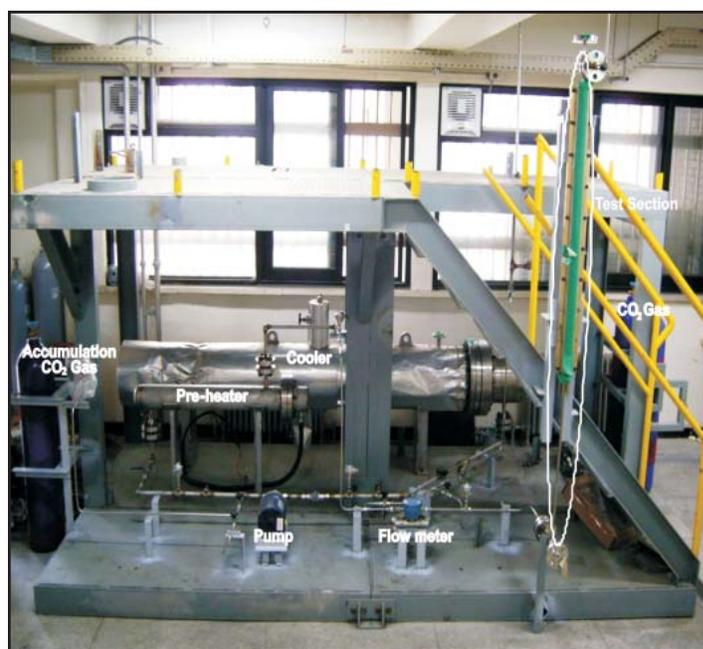
Figure 1. Test apparatus for measurement of heat transfer coefficients for supercritical CO<sub>2</sub>.
