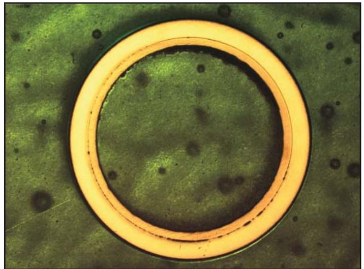
Figure 2. Zr-lined HT-9 cladding tube fabricated using a plug-drawing process.
