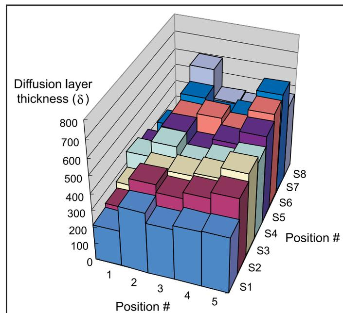
Figure 3. Calculated diffusion layer thicknesses on the cathode side wall.
