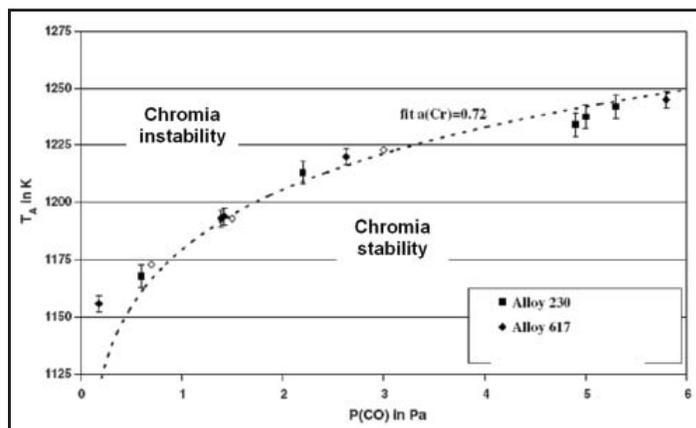
Figure 1. Critical temperature for the chromia stability versus CO partial pressure in helium; the open symbols represent Inconel 617 from the literature.
