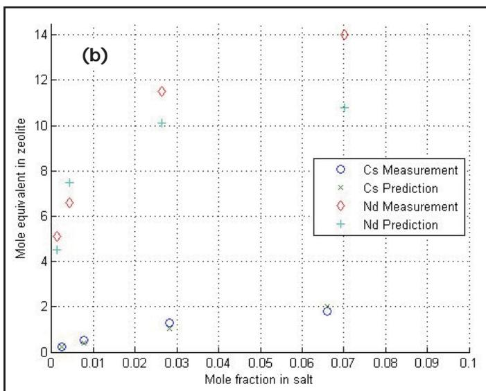
Figure 1b. LiCl-KCl-CsCl-NdCl<sub>3</sub> measurements and predictions.
