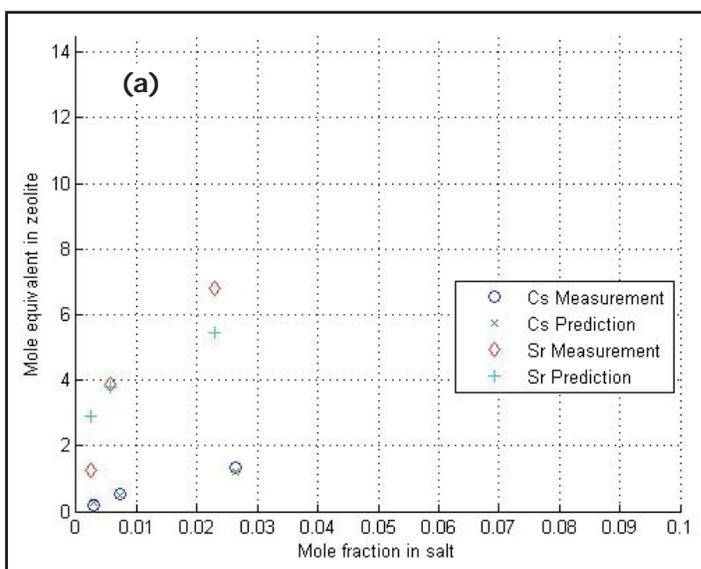
Figure 1a. Quaternary salts LiCl-KCl-CsCl-SrCl<sub>2</sub> measurements and predictions.
