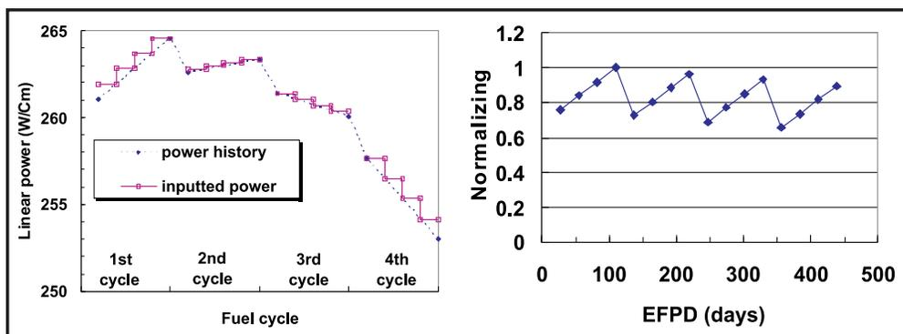
Figure 1. Linear power for the MACSIS input.
