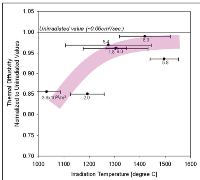
Figure 3. Thermal diffusivity of neutron-irradiated ZrC normalized to non-irradiated values. The horizontal error bars correspond to uncertainty of irradiation temperature.
