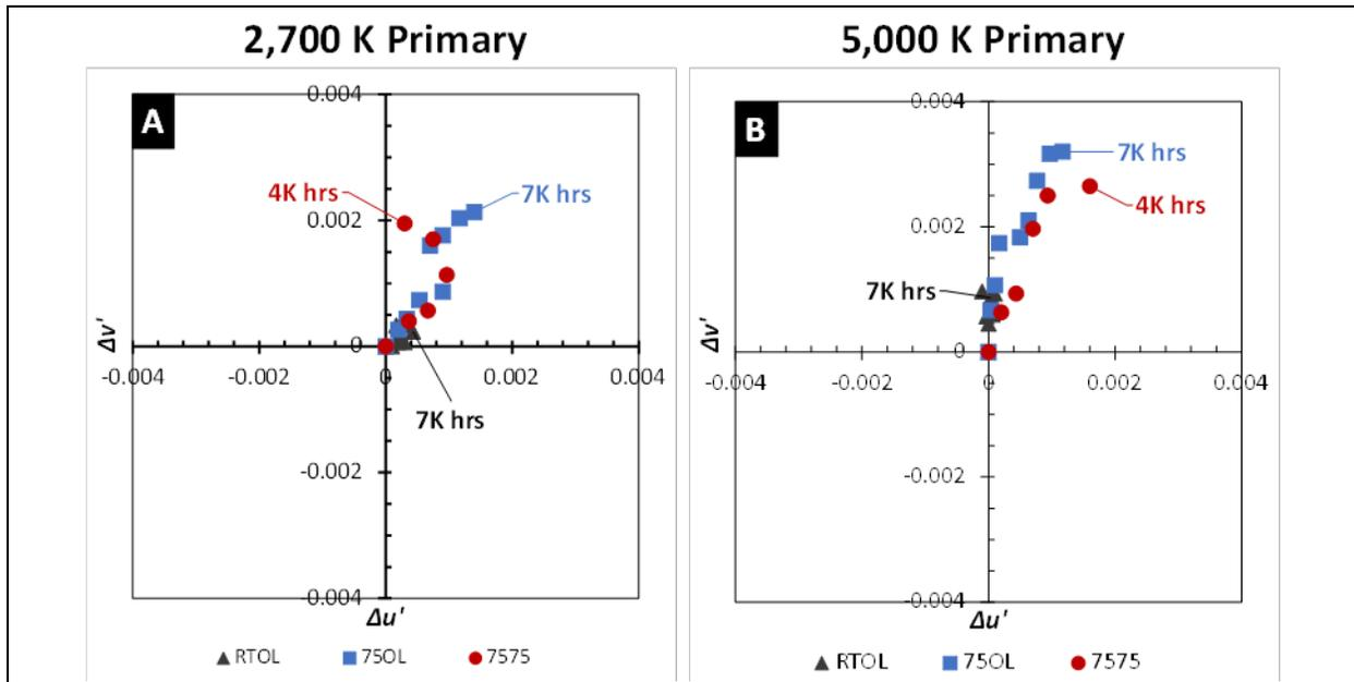
Figure 3-23: Chromaticity shift for Product MS-4: (A) for the 2,700 K primary and (B) for the 5,000 K primary.
