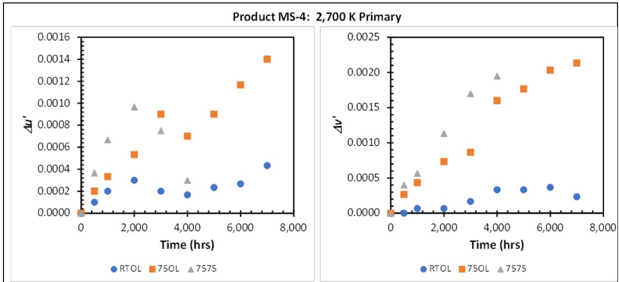
Figure A-9: Temporal change in  $\Delta u'$  and  $\Delta v'$  from the 2,700 K primary of Product MS-4 in different AST environments.
