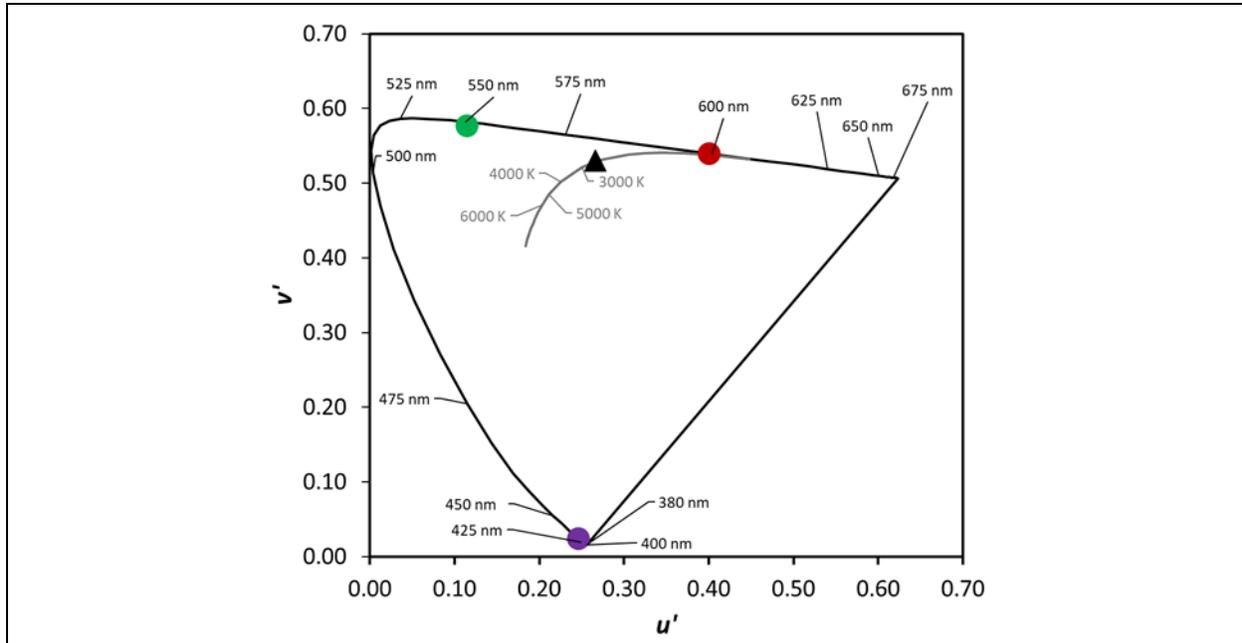
Figure 3-11: Chromaticity coordinates of the violet, green, and red emitters used in Product MS-2 plotted on the 1976 CIE chromaticity diagram. The black triangle is the chromaticity point of the white light produced by Product MS-2.
