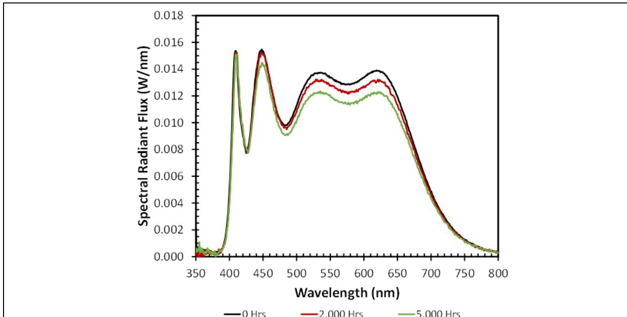
Figure 3-16: SPDs for Product MS-3 operated during 75OL for various times.
