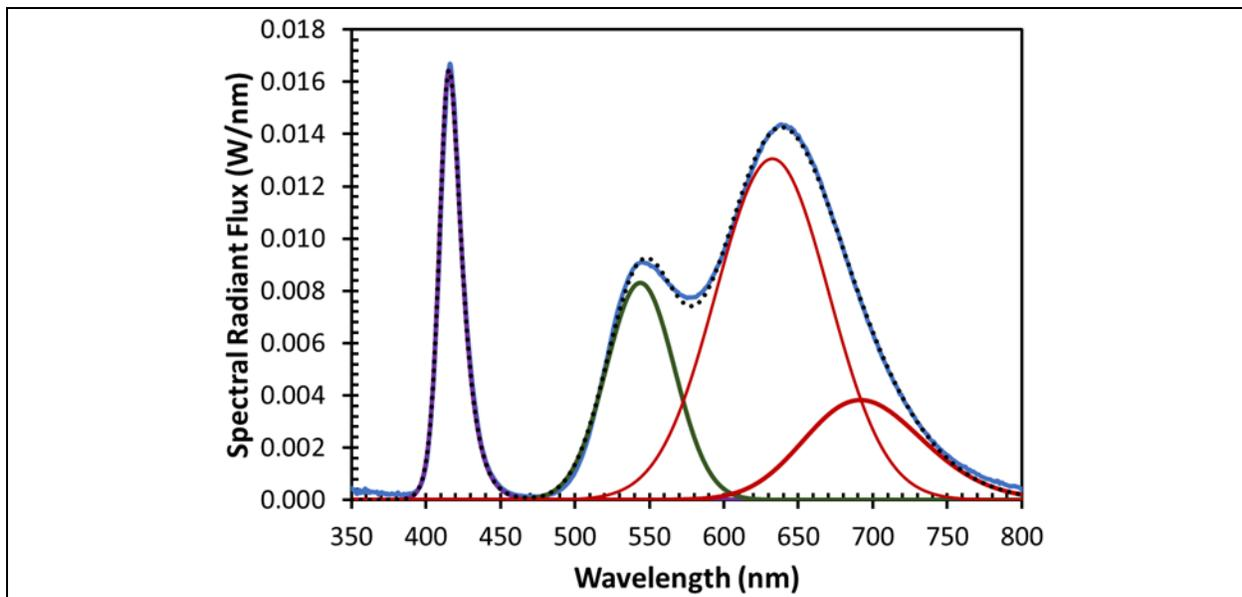
Figure 3-10: Spectral deconvolution of the initial emissions from Product MS-3.
