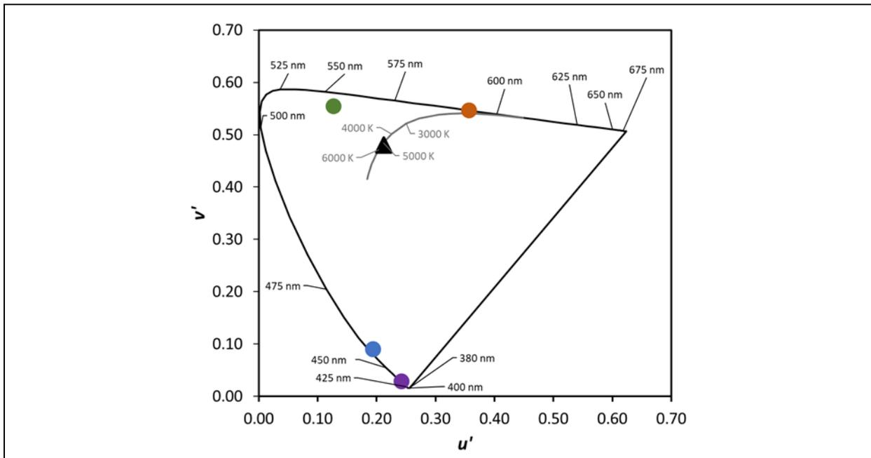
Figure 3-19: Chromaticity coordinates of the violet, blue, green, and orange-red emitters used in Product MS-3 are plotted on the 1976 CIE chromaticity diagram. The black triangle is the chromaticity point of the white light produced by Product MS-3.
