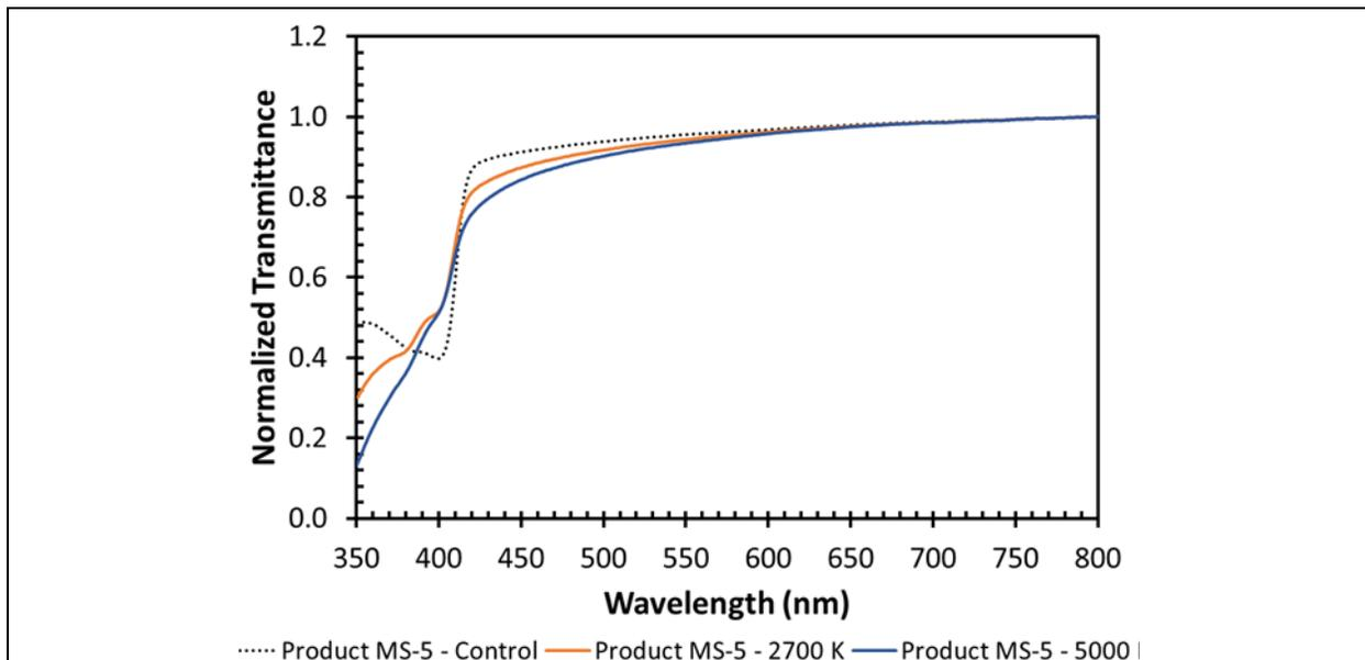
Figure 3-31: Transmittance data (normalized at 800 nm) for Product MS-5 lenses show less transmittance at high energy wavelengths after AST.
