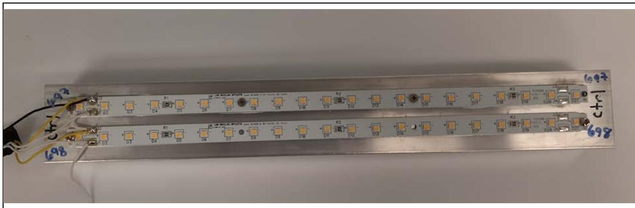
Figure 2-5: Product MS-3 LED light engine consisting of two LED modules mounted on a common heat sink.
