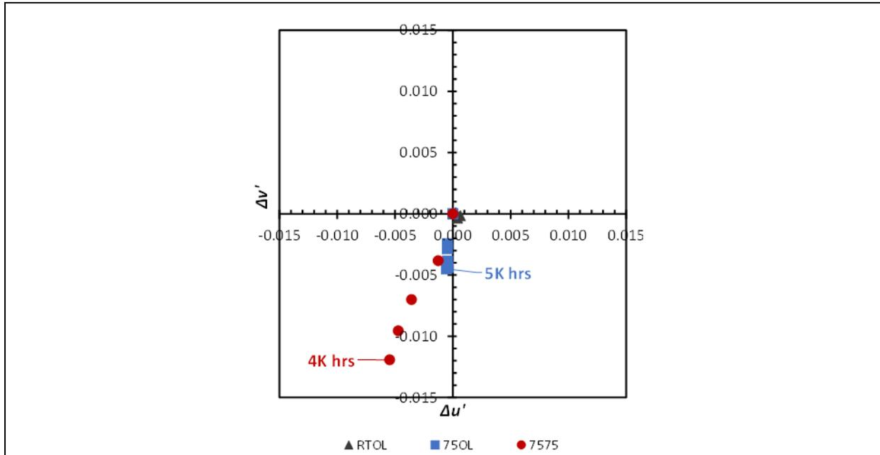
Figure 3-15: Chromaticity shift diagram for Product MS-3 in RTOL, 75OL, and 7575.
