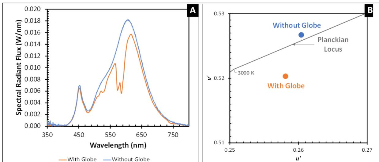
Figure 2-3: A comparison of light emission from Product MS-1 with and without the glass globe. (A) SPDs of Product MS-1 with the glass globe (orange trace) and without the globe (blue trace), and (B) chromaticity coordinates with the globe (orange) and without the globe (blue).
