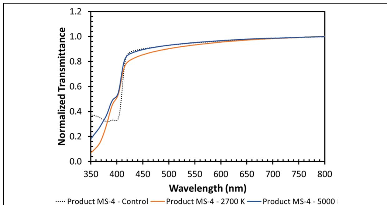
Figure 3-25: Transmittance data (normalized at 800 nm) for Product MS-4 lenses show less transmittance at high energy wavelengths after AST.
