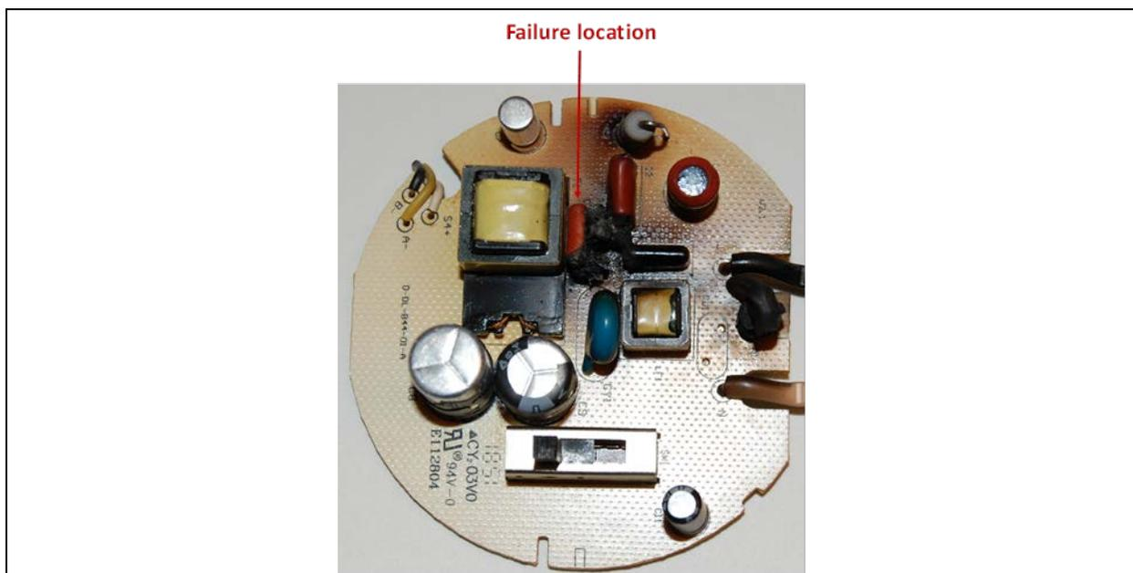
Figure 3-24: Failed driver from Product MS-4 after 5,000 hrs of 7575.
