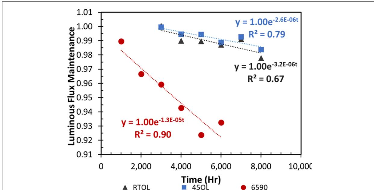
Figure 3-6: LFM of Product MS-2 during RTOL, 45OL, and 6590 according to IES LM-84-14 and IES TM-28-14.
