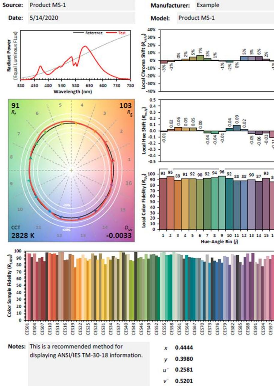
Figure A-1. ANSI/IES TM-30-18 analysis for Product MS-1 with the glass globe.
