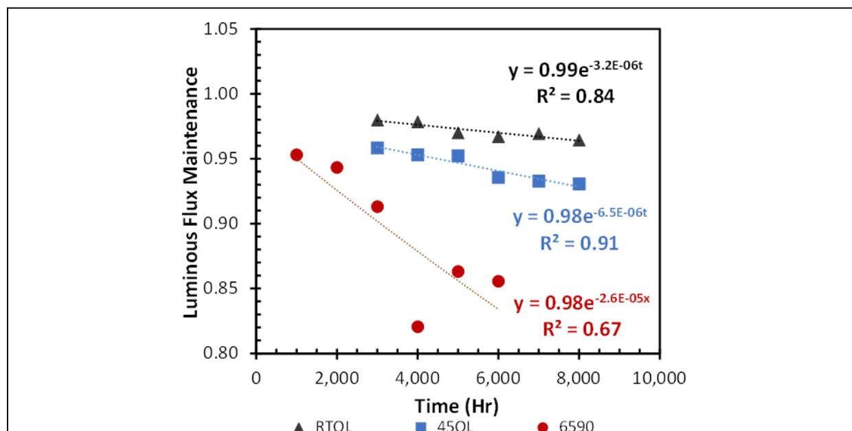
Figure 3-1: LFM of Product MS-1 during RTOL, 45OL, and 6590 according to IES LM-84-14 and IES TM-28-14.
