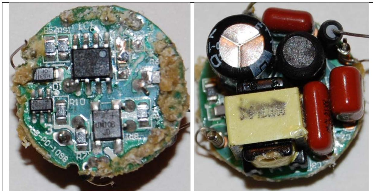
**Figure 2-2:** Front (on left) and back (on right) views of the driver used with Product MS-1.
