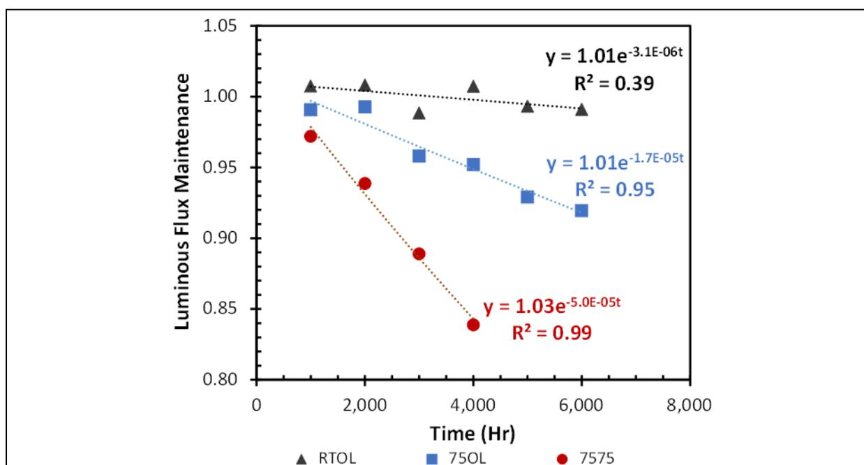
Figure 3-27: LFM of the 5,000 K primary for Product MS-5 in different AST protocols.
