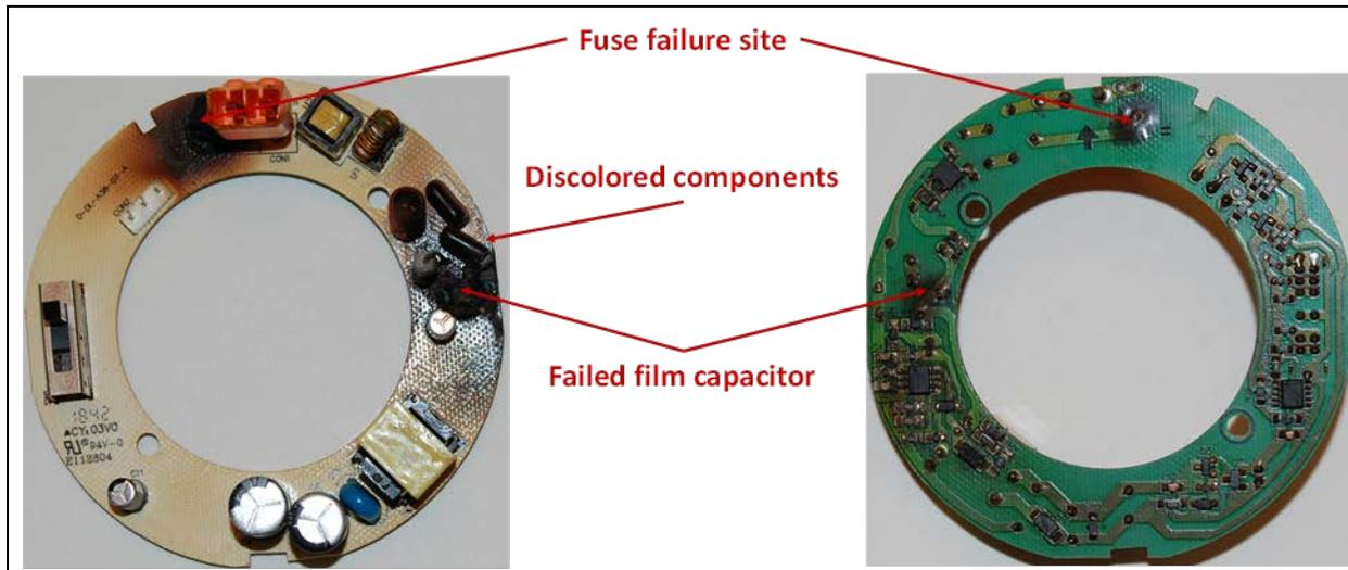
Figure 3-30: Failed driver from Product MS-5 after 5,000 hrs of 7575.
