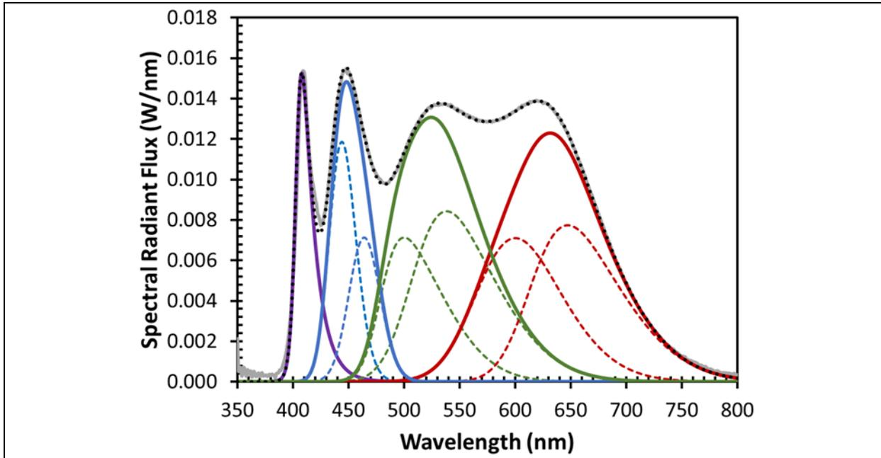
Figure 3-18: Spectral deconvolution of the initial emissions from Product MS-3.
