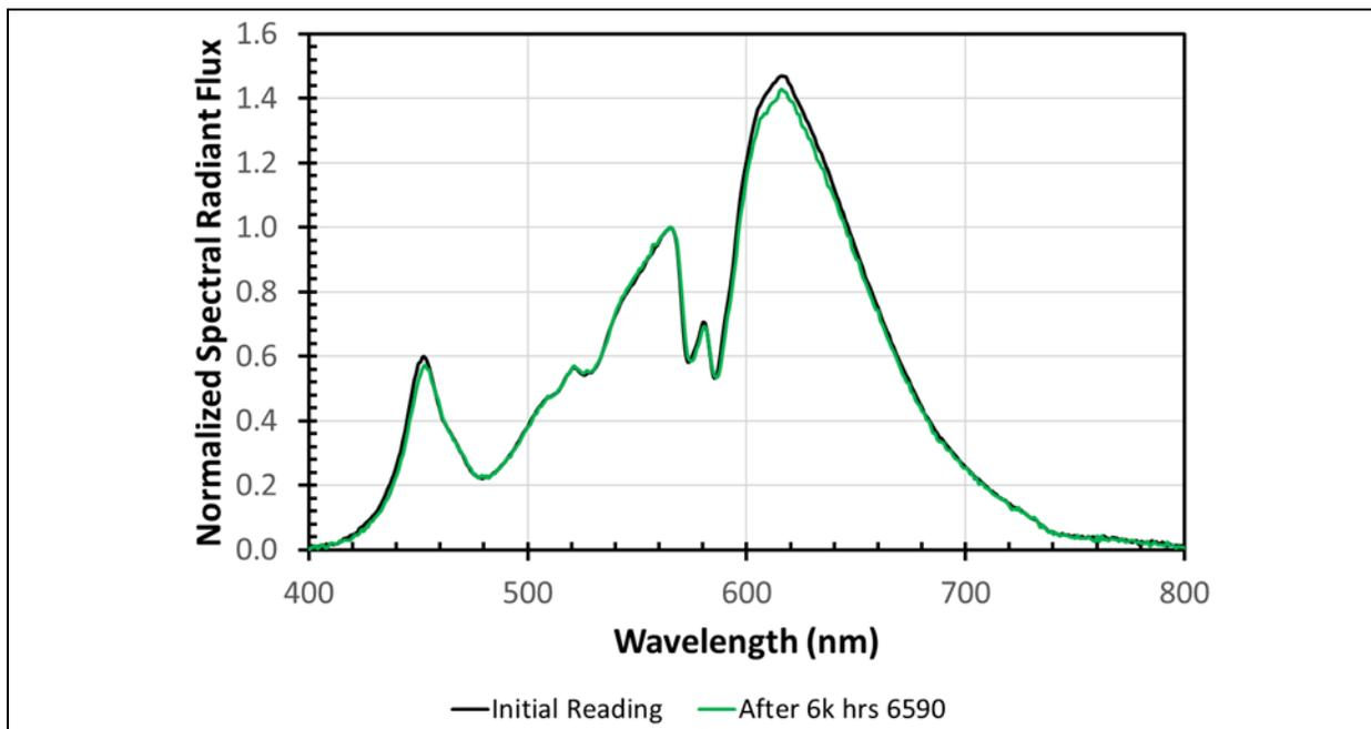
**Figure 3-4:** Normalized radiant flux for Product MS-1 at the beginning of testing and after 6,000 hrs of exposure during 6590. Spectra were normalized to the green emission peak at 565 nm.
