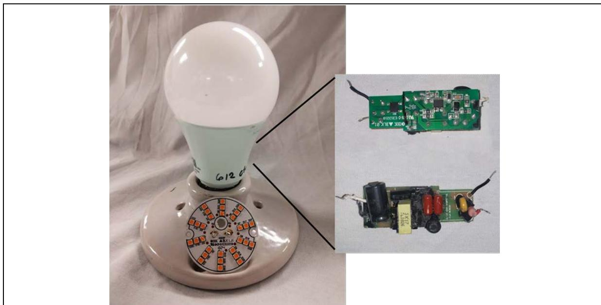
Figure 2-4: (On left) Product MS-2 with the globe, but in an unenergized state, along with the LED module. (On right) A close-up image of the driver used in Product MS-2.
