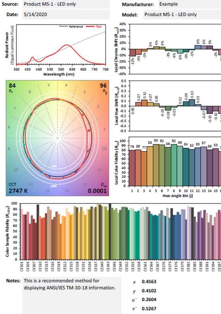
Figure A-2: ANSI/IES TM-30-18 analysis for LEDs from Product MS-1 without the glass globe.
