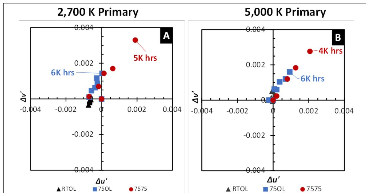
Figure 3-29: Chromaticity shift for Product MS-5: (A) for the 2,700 K primary and (B) for the 5,000 primary.
