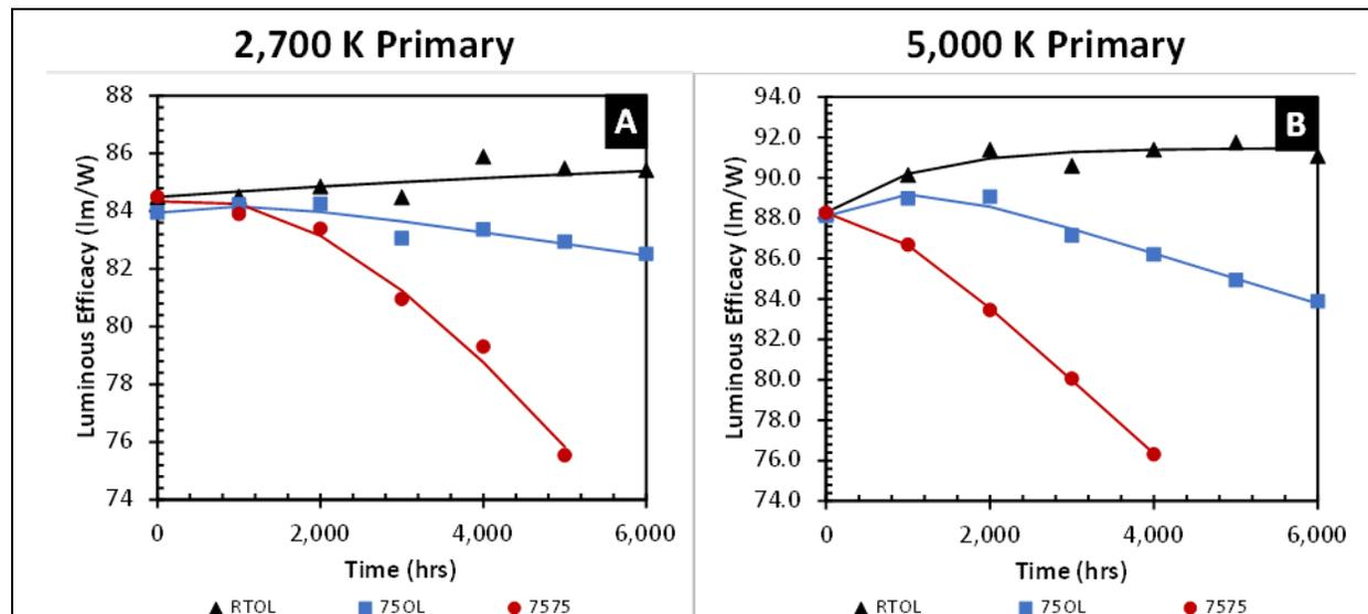
Figure 3-28: Temporal change in luminous efficacy for Product MS-5: (A) for the 2,700 K primary and (B) for the 5,000 primary.
