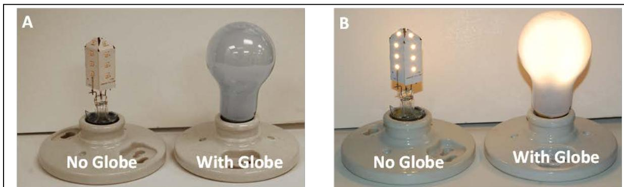
**Figure 2-1.** Product MS-1 without the globe and with the globe. (A) Lamps in unenergized state and (B) lamps energized with ac power.
