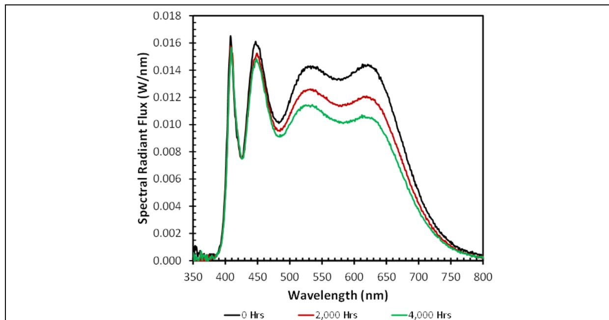
**Figure 3-17: SPDs for Product MS-3 operated during 7575 at various times.**
