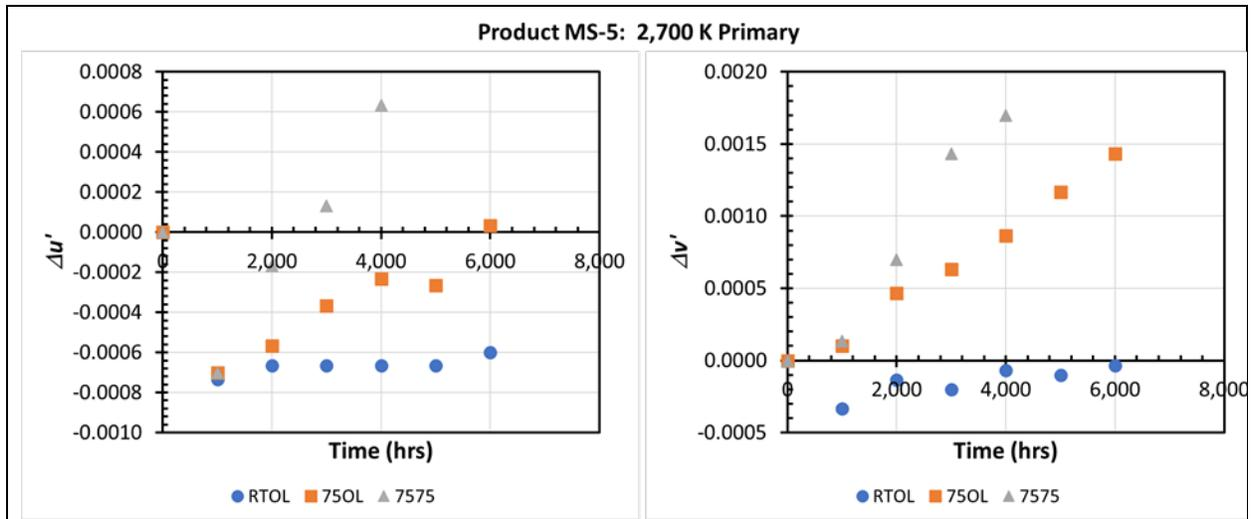
Figure A-11: Temporal change in  $\Delta u'$  and  $\Delta v'$  from the 2,700 K primary of Product MS-5 in different AST environments.
