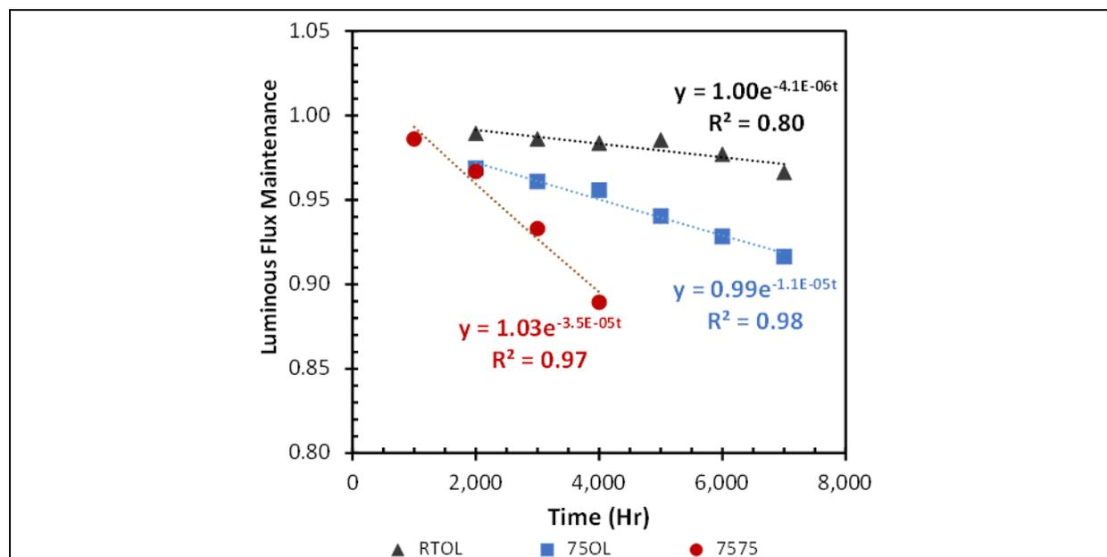
Figure 3-20: LFM of the Product MS-4 test populations operated with the 2,700 K primary. Testing was performed during RTOL, 750L, and 7575.
