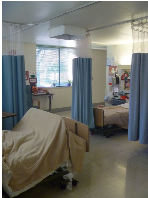
Figure 10. Photo of one four-bed resident room during the day. Note the over-bed light with upward light only.
