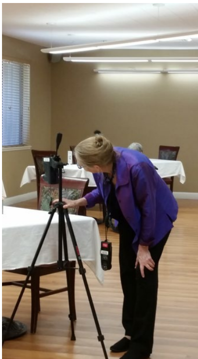
Figure 13. Photo of tripod set up in ACC dining room. The spectrometer was mounted to take vertical measurements at a height of 42", the eye height of a typical resident in a wheelchair.
