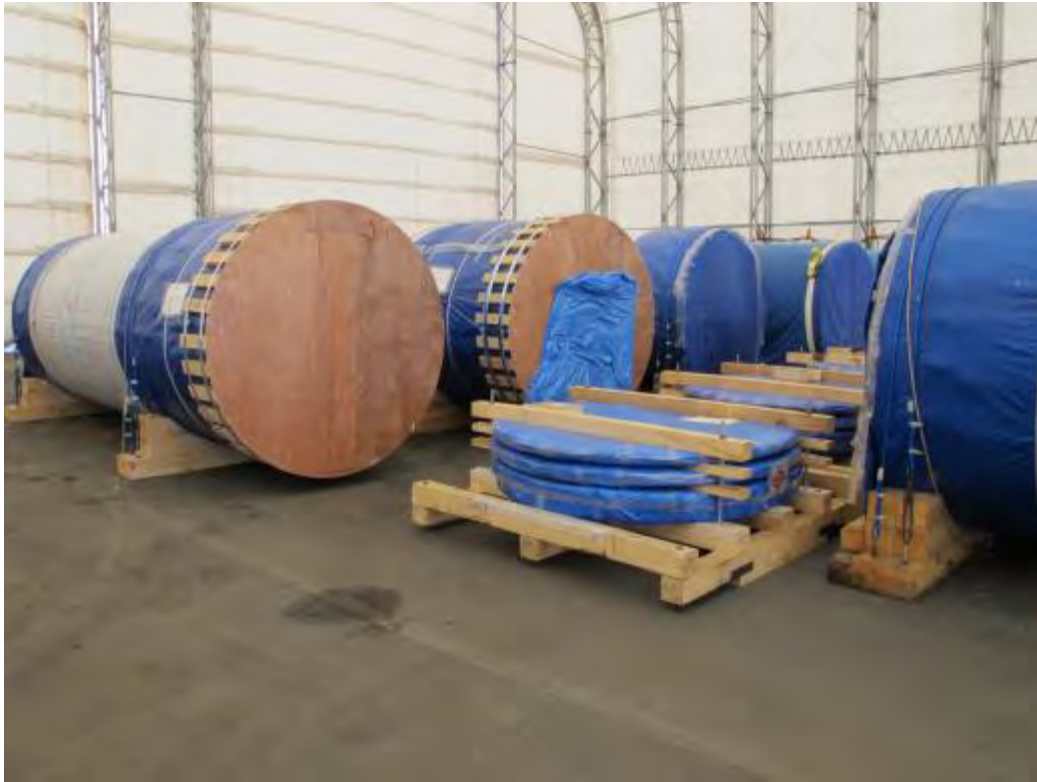
Figure 2-260. 32PTH2 Dry Storage Canisters (On Left) (2015)
