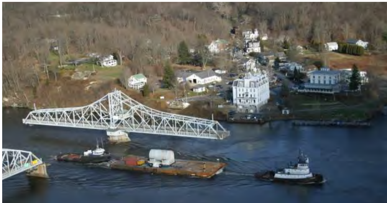
Figure 2-42. Connecticut Yankee Reactor Pressure Vessel Being Transported on Barge in the Connecticut River
