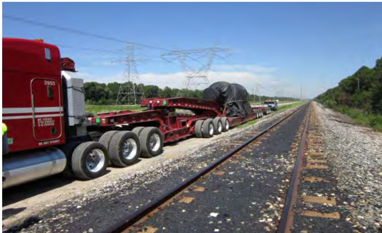
Figure 2-194. High Pressure Turbine Rotor Delivered to Crystal River Site by Heavy Haul Truck (2011)
