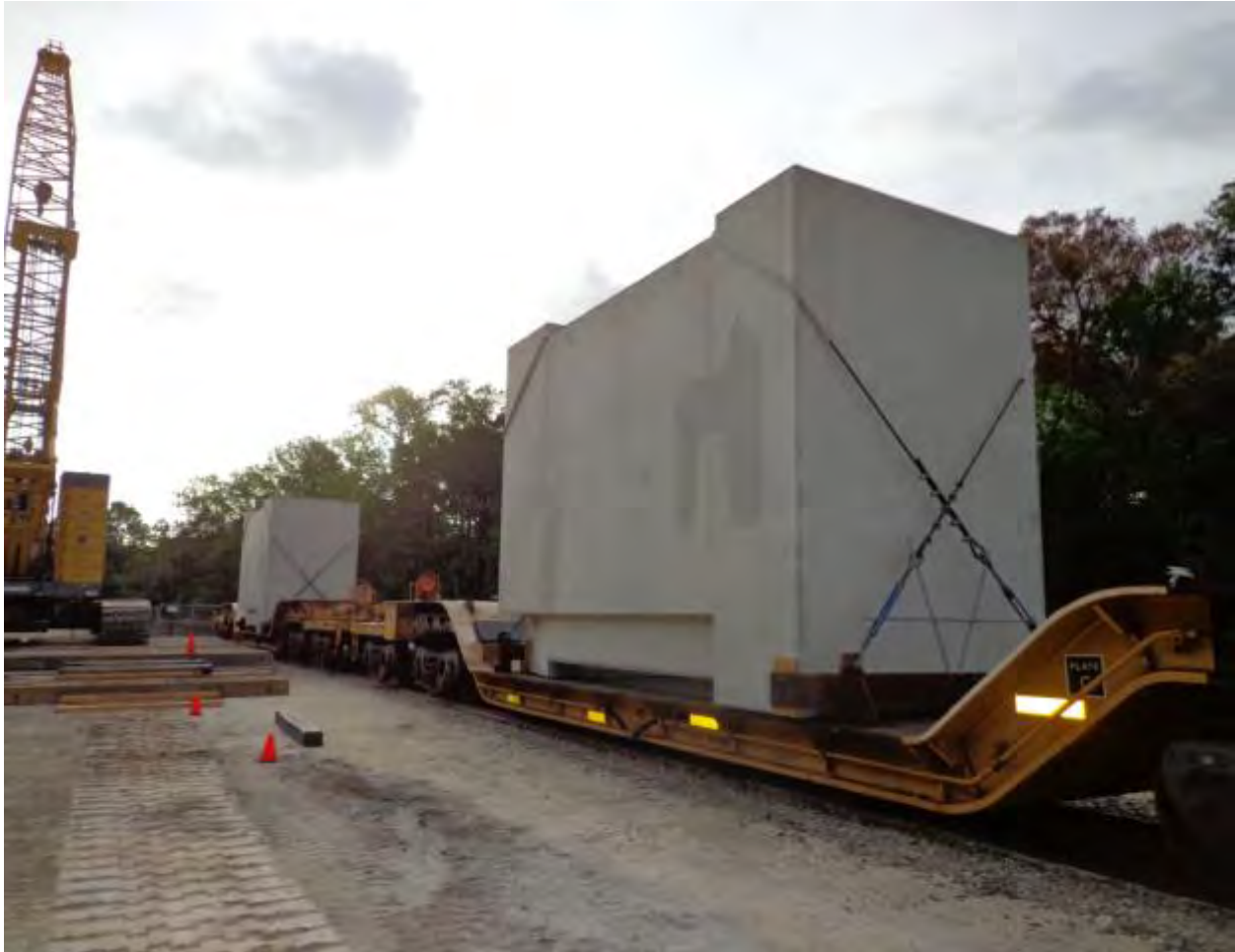
Figure 2-181. Two Horizontal Storage Modules Loaded on Railcars (2015)
