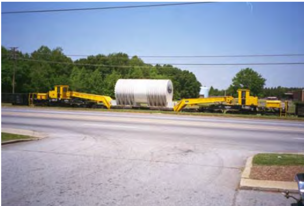
Figure 2-27. Yankee Rowe Reactor Pressure Vessel on Railcar (1997)
