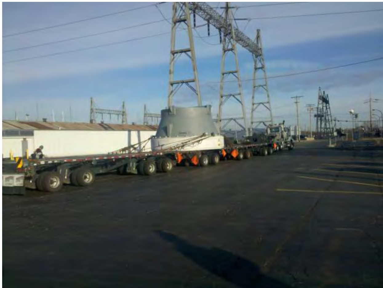
Figure 2-146. Zion Reactor Head on Heavy Haul Truck Transporter (2011)
