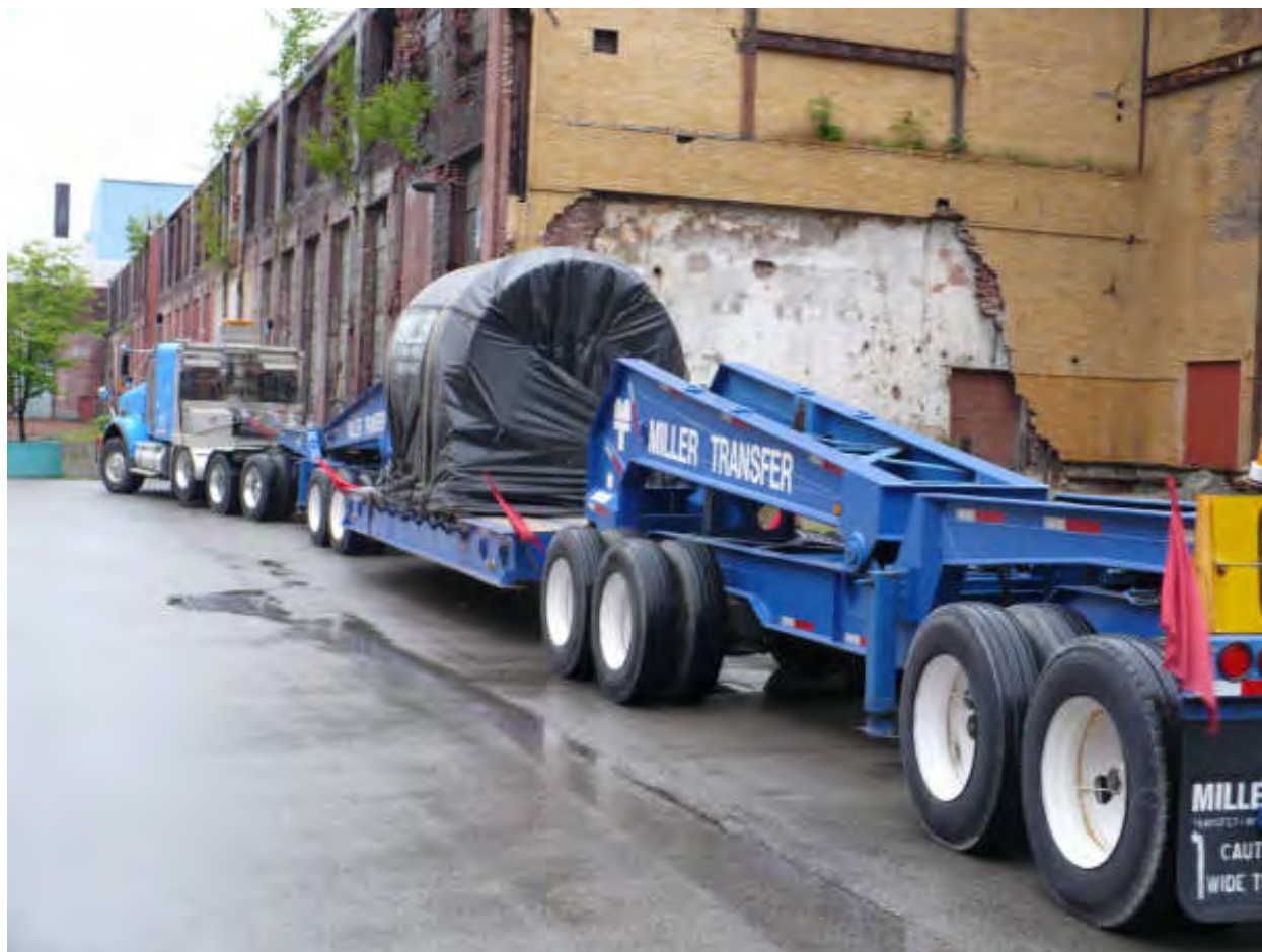
Figure 2-47. Empty HI-STAR HB Cask Being Transported by Heavy Haul Truck
