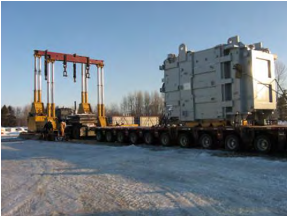
Figure 2-209. Gantry System Used to Transfer Transformers from Railcars to Goldhofer Trailers (2008)
