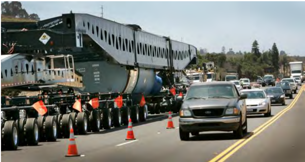
Figure 2-294. Old Steam Generator on Heavy Haul Truck Transporter (2011)
