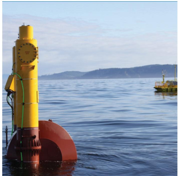
Northwest Energy Innovations verified the ocean wavelength functionality of the Azura device (previously called WET-NZ) through wave tank testing and a controlled open-sea deployment of its 1:2 scale device.
