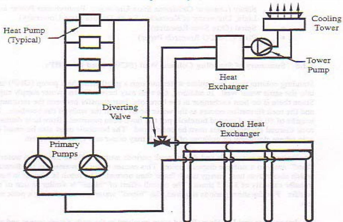
Figure 1.3 Hybrid System Using A Cooling Tower
