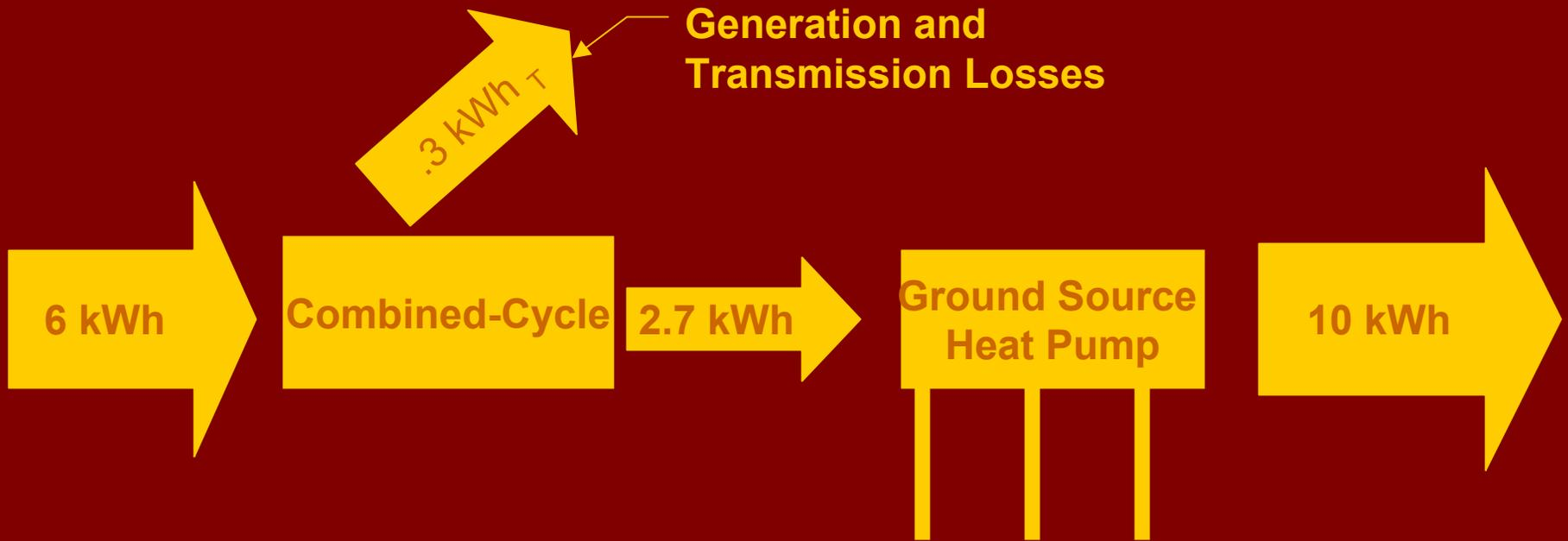
Generation efficiency approaches 55% compared with 35% for a steam cycle alone. GSHP require only 6 kWh<sub>T</sub> from the source to provide 10 kWh<sub>T</sub> to the building due to the increase in power plant efficiency.
