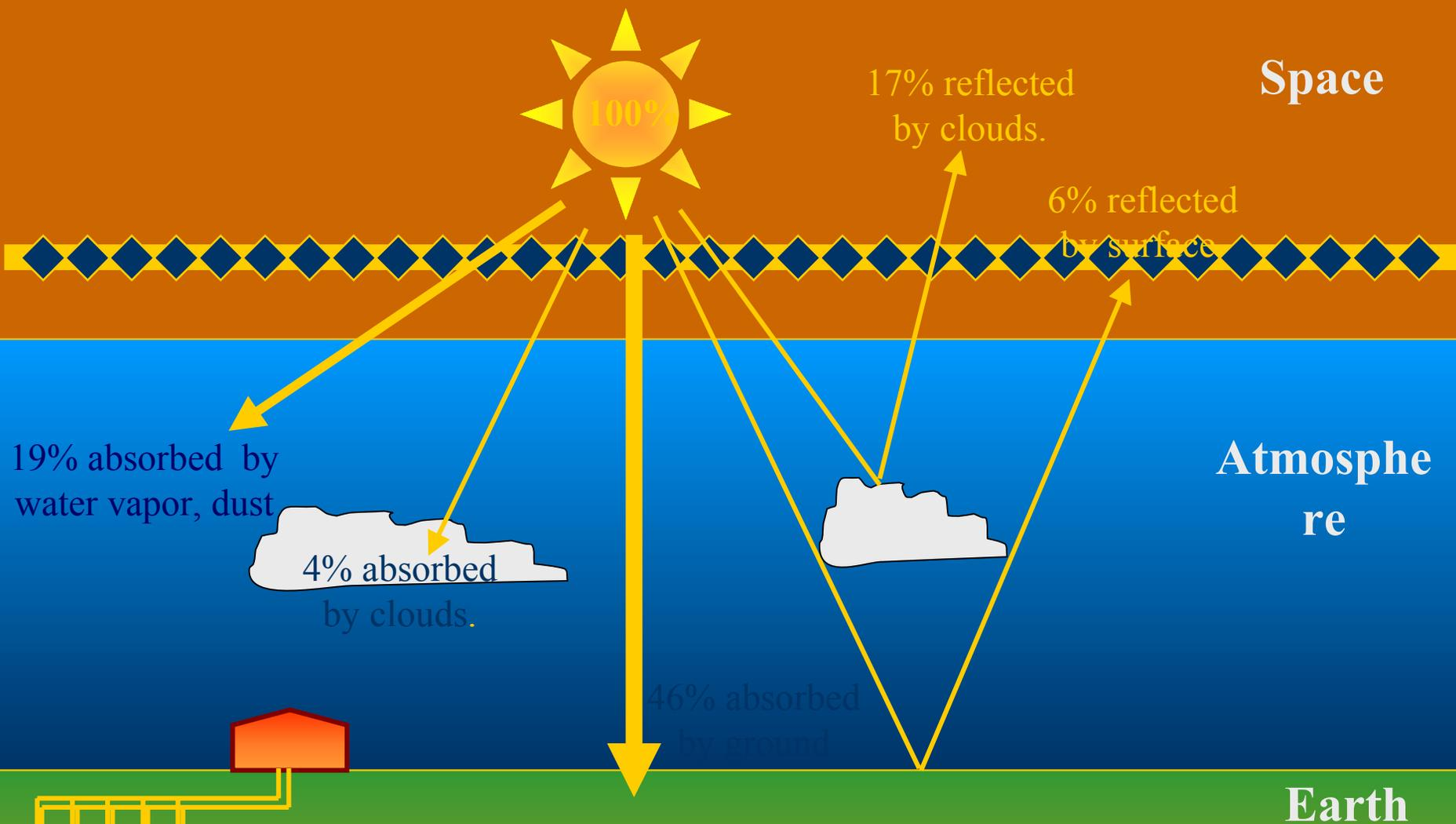
The earth is like a solar battery absorbing nearly half of the sun's energy. The ground stays a relatively constant temperature through the seasons, providing a warm source in winter & a cool heat sink in summer.
