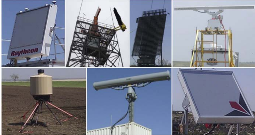
Figure 1. Several wind turbine radar interference approaches tested in the IFT&E campaigns (clockwise from top left: Raytheon X-band Radar; Booz Allen Hamilton canceling post; Lockheed TPS-77 Radar; C-Speed Lightwave Radar; SRC LSTAR Radar; Terma Scanter 4002 Radar; and Aveillant Holographic Radar)
