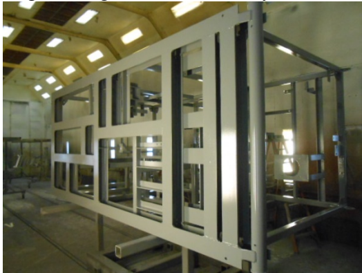
Skid in paint booth
