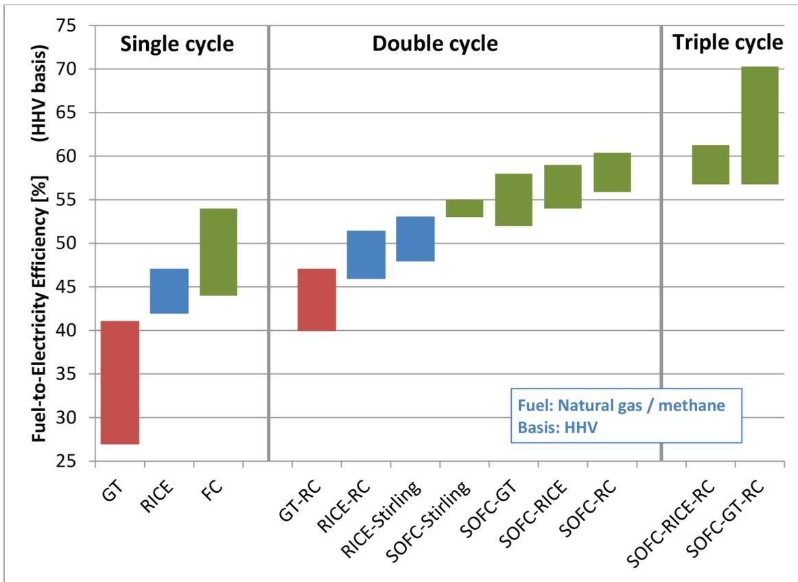
Key: GT = gas turbine; RICE = reciprocating internal combustion engine; FC = fuel cell (molten carbonate or solid oxide); SOFC = solid oxide fuel cell. The Appendix provides background on how these efficiencies were calculated.
