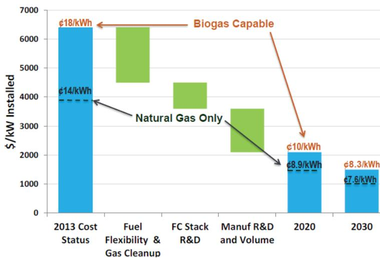
Figure 4.Q.4 shows the R&D waterfalls chart for CHP fuel cells on natural gas and biogas.
