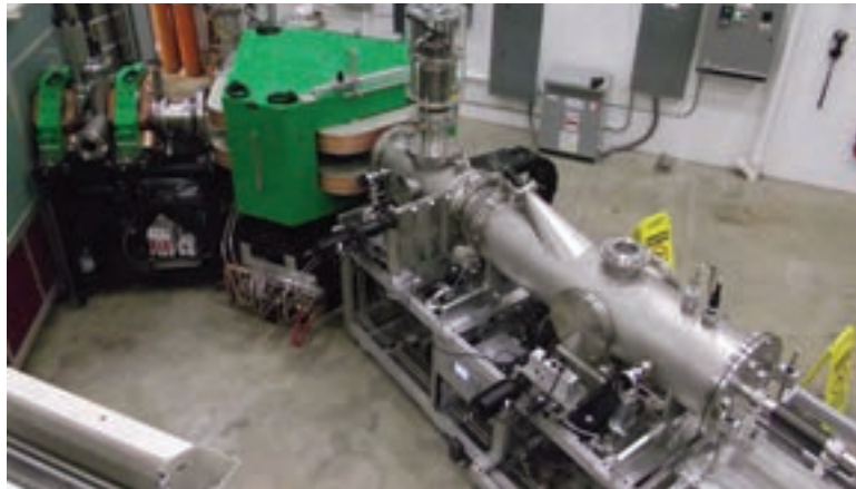
Figure 9.20 The EMIS for Stable Isotope Enrichment at ORNL
