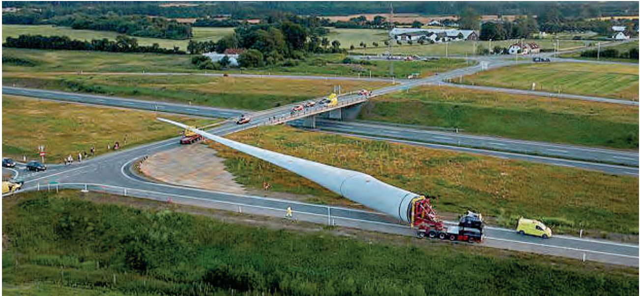
Figure 5-11. Transport of Large Wind Turbine Blade 105
