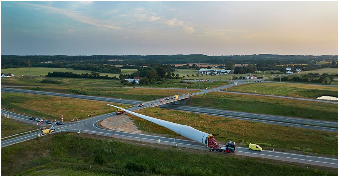
Figure 5-4. Example of wind turbine blade transportation obstacles
