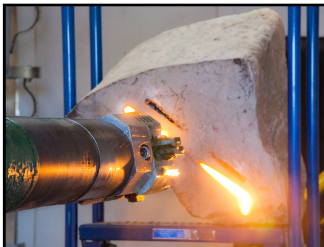
A patented laser technology is performing at commercial strength in the laboratory. The tool has been adapted for harsher geothermal downhole settings and will be field tested next year. Source: Foro Energy
