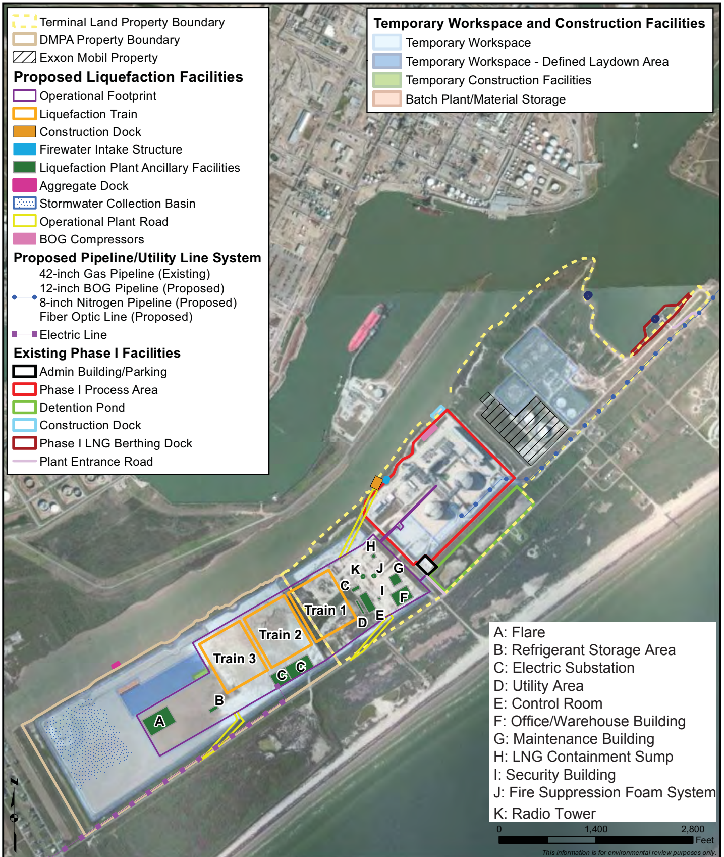
Figure 1-2 Freeport LNG - Liquefaction Project Proposed Liquefaction Facilities and Workspace Layout at and Adjacent to Quintana Island Terminal Brazoria County, Texas
