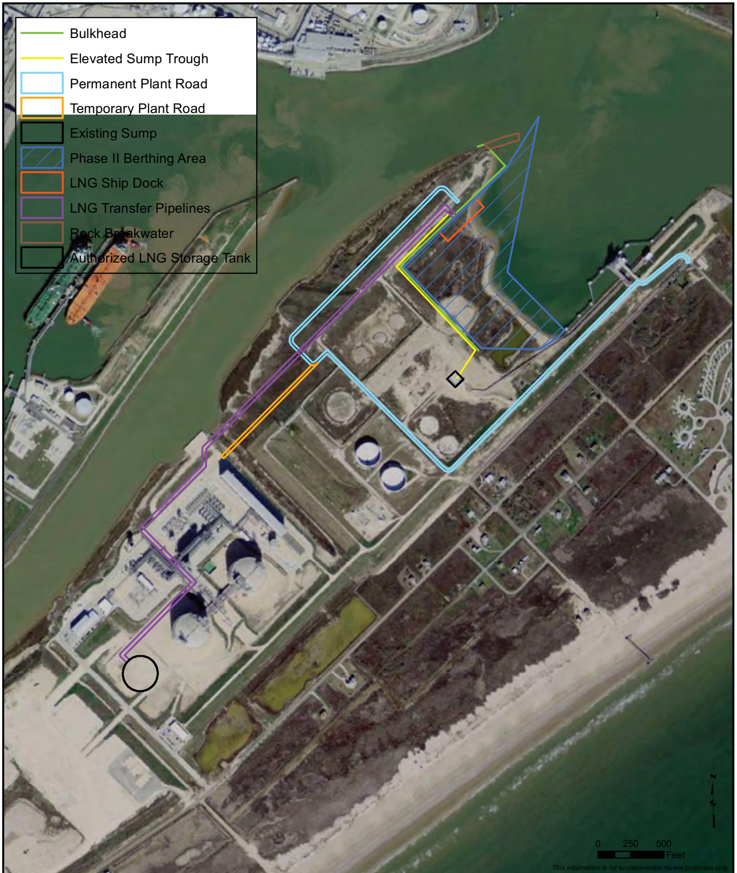
Figure 1-4 Freeport LNG - Phase II Modification Project Proposed Facilities and Components at the Quintana Island Terminal Brazoria County, Texas
