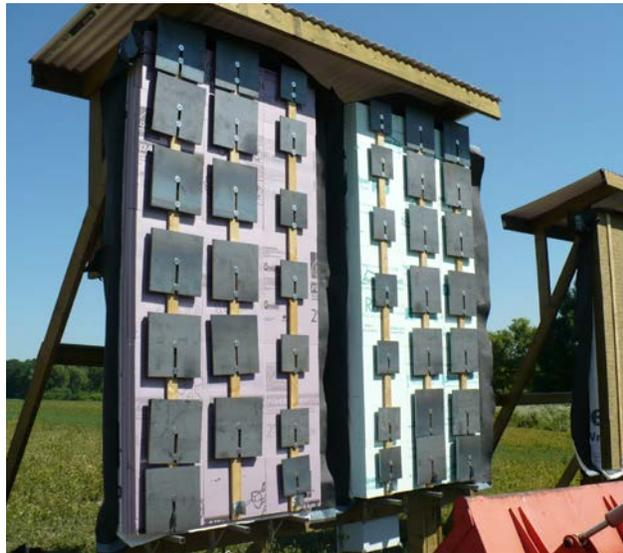
Exterior environmental exposure testing examined four types of insulation materials. Each test panel was constructed with two layers of 2 in. thick insulation, and loaded to three different load magnitudes (8 lbf, 15 lbf, and 30 lbf per fastener). The vertical movement of the furring strip (downward and upward) was recorded over a period of approximately 450 days.
