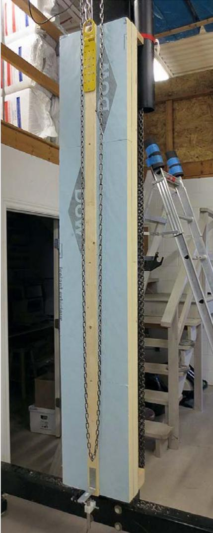
Full-scale assemblies were used to limit variations in installation from affecting the test results. Over the course of the testing, several test iterations were completed that varied insulation type and fastener spacing.
