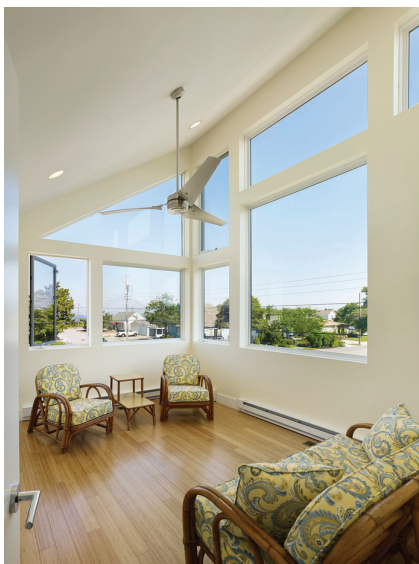
Large north-facing windows provide daylight and views without adding much solar heat gain.
