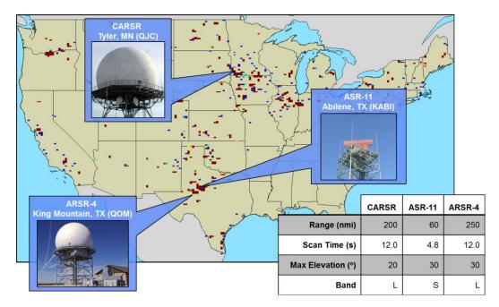
**Test 1:** The first campaign took place in April 2012. The purpose of the first test was to characterize the performance of a newly upgraded Common Air Route Surveillance Radar (CARSR), a long range surveillance radar system, in Tyler, MN. Three private sector companies that demonstrated their mitigation systems were: the C Speed Lightwave in-fill radar, the SRC LSTAR(V)3 in-fill radar, and the Raytheon Long Range Radar processing upgrade.
