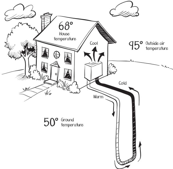
The average underground temperature of the soil (10' down) is 45°-55°F (7°-13°C). In winter, a geothermal heat pump brings the earth's natural warmth up to your house and then transfers it into each room. In summer, the system works in reverse to supply air conditioning by absorbing the heat from inside the home and transferring it to the cooler earth below.
