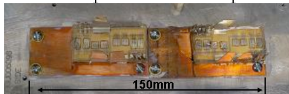
Two 100A/1200V SiC Power Modules in a HF converter (liquid cooled)
