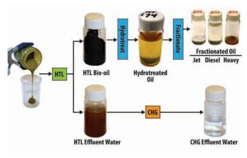
Figure 20. The process flows of HTL and HTL with CHG.
