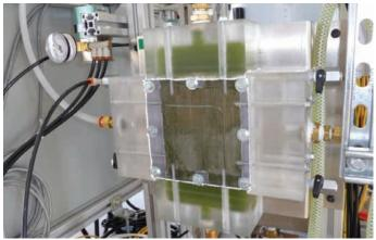
Figure 17. Cross-flow membrane modules assembled for field tests (0.26 m<sup>2</sup> of membrane area, 1 mm feed flow channel opening).
