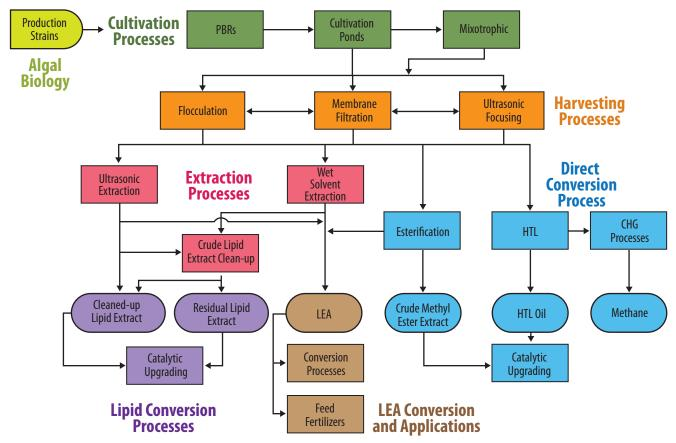
Figure 4. The NAABB Process Matrix.
