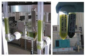
Figure 16. Ultrasonic harvester. Left panel, side view of two 2 L modules attached to a customized cart containing twelve modules. The dilute feedstock is fed into the modules by gravity flow and the concentrate is collected from the bottoms of the modules. Right panel, visual comparison of the dilute feedstock (left tube) and concentrated product (right tube).
