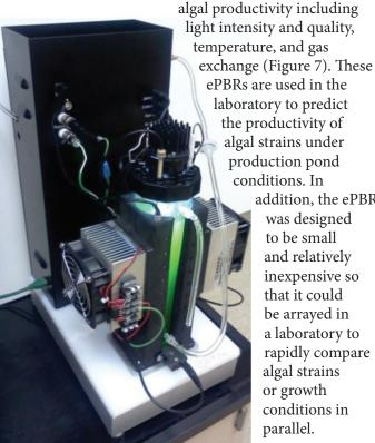
Figure 7. The Environmental Photobioreactor (ePBR).
