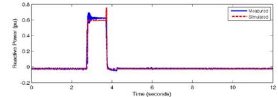
Modeled and measured comparison of a type 3 WTG response to a voltage dip at high side of step-up transformer.
