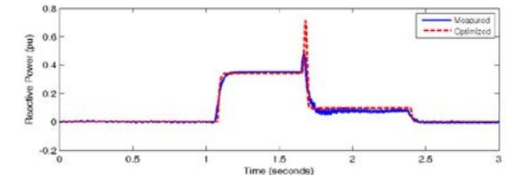
Modeled and measured comparison of a type 4 WTG response to a voltage dip at high side of step-up transformer.
