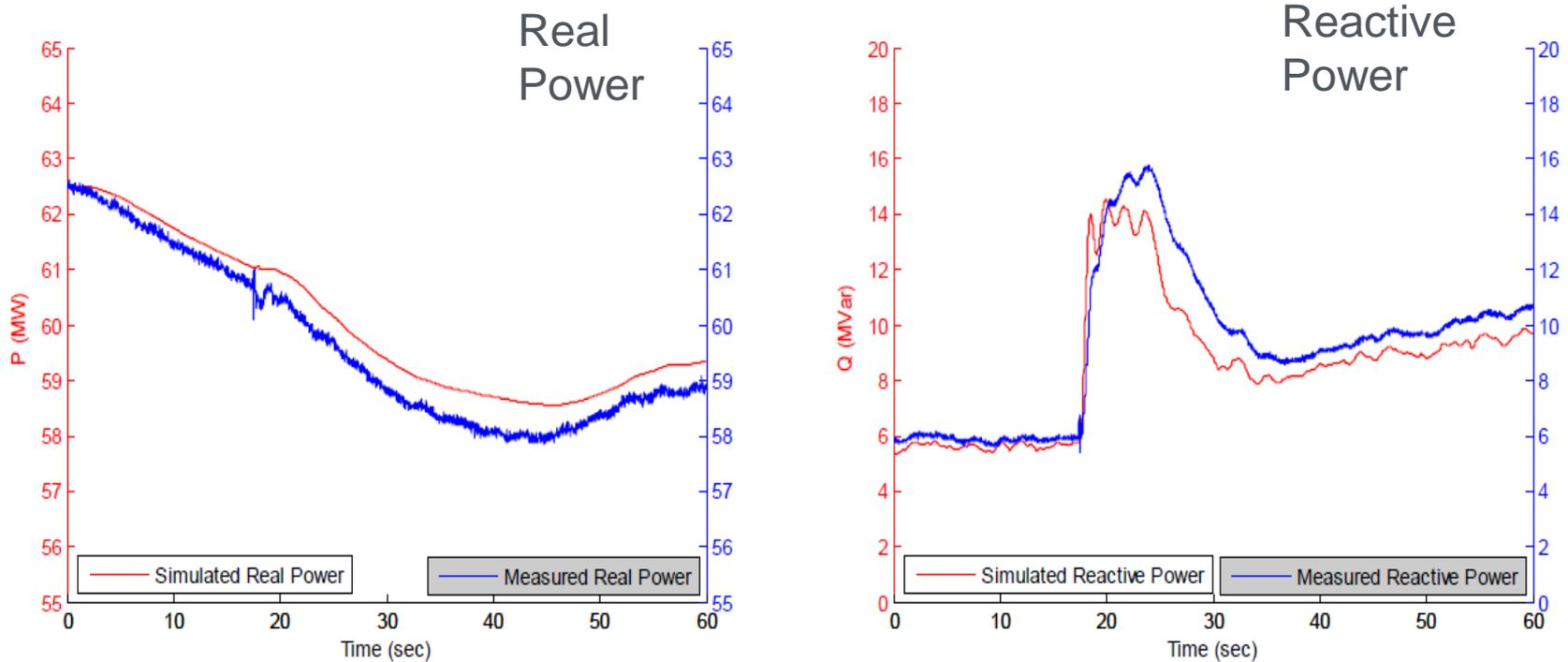
An example of dynamic model validation (**measured** data vs. **simulated** data)
