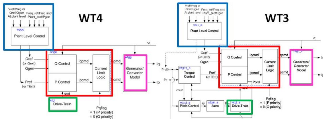
Block diagram of type 3 and type 4 WTG models
